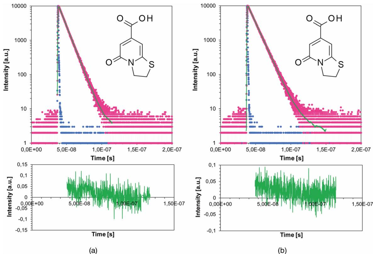
Fig. 5 Fluorescence lifetimes measurements conducted for CCA fluorophore in (a) distilled water and (b) acetonitrile showing sample's decay, reference and model fit used to calculate the precise fluorescence lifetimes along with model residuals obtained for each of the curves respectively.
