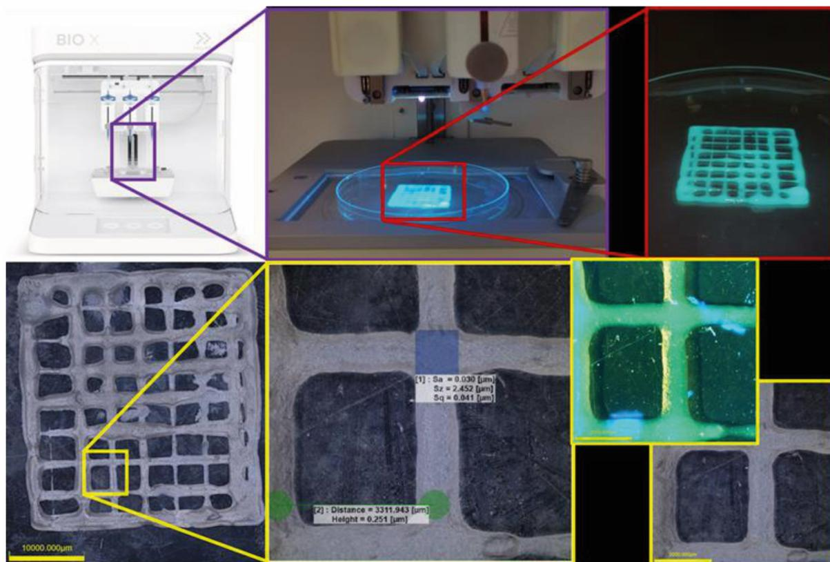
**Fig. 14** Microscopic images of obtained 3D prints manufactured using BioX™ printer equipped with a diode of a wavelength of 405 nm and intensity at the sample of  $9.88 \text{ mW cm}^{-2}$  using a composition consisting of poly(ethylene glycol)diacrylate (70 wt%) and poly(ethylene glycol) (30 wt%). The photoinitiating system consisted of (1.0 wt%) of IOD and (0.1 wt%) of CCA fluorophore.
