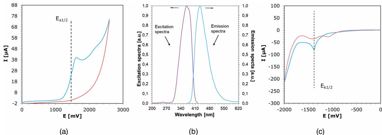
**Fig. 4** (a) Cyclic voltammetry for oxidation process (CVox, vs. Ag/AgCl) experiments in ACN (containing 0.1 M tetrabutylammonium hexafluorophosphate) for CCA; (b) excitation and emission spectra for the determination of the excited singlet state energy for CCA for the solution in acetonitrile; (c) cyclic voltammetry for reduction process (CVred, potential vs. Ag/AgCl) experiments in ACN (containing 0.1 M tetrabutylammonium hexafluorophosphate) for CCA.
