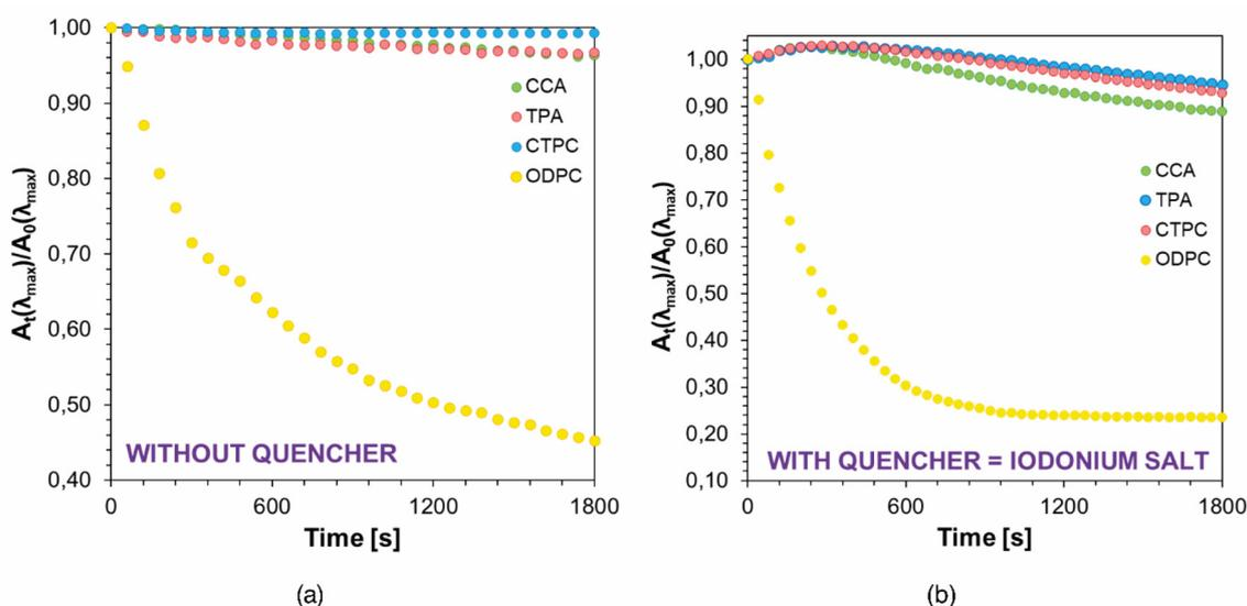
**Fig. 8** Photo-decomposition of (a) all of the chromophores in acetonitrile and (b) the same solutions with the addition of IOD ( $1.86 \times 10^{-4} \text{ mol dm}^{-3}$ ) carried out for 30 minutes during irradiation with 405 nm UV-LED at 1.0 A (1000 mW cm<sup>-2</sup>) shown as the corresponding absorbance correlation at the absorbance maximum ( $\lambda_{max}$ ).
