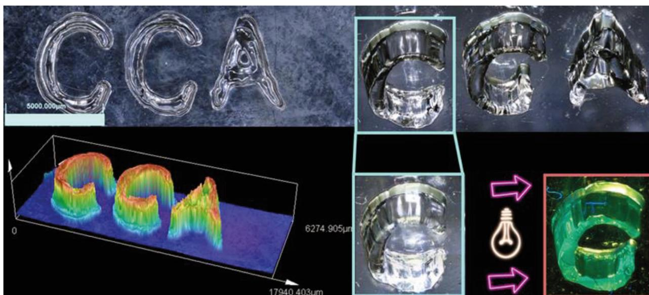
**Fig. 13** Microscopic images of obtained 3D prints manufactured using laser engraver printer machine (NEJE DK-8-KZ) equipped with a laser of a wavelength of 405 nm and intensity of 1500 mW using a composition consisting of poly(ethylene glycol)diacrylate (70 wt%) and water (30 wt%). The photoinitiating system consisted of (1.0 wt%) of IOD and (0.1 wt%) of CCA fluorophore.
