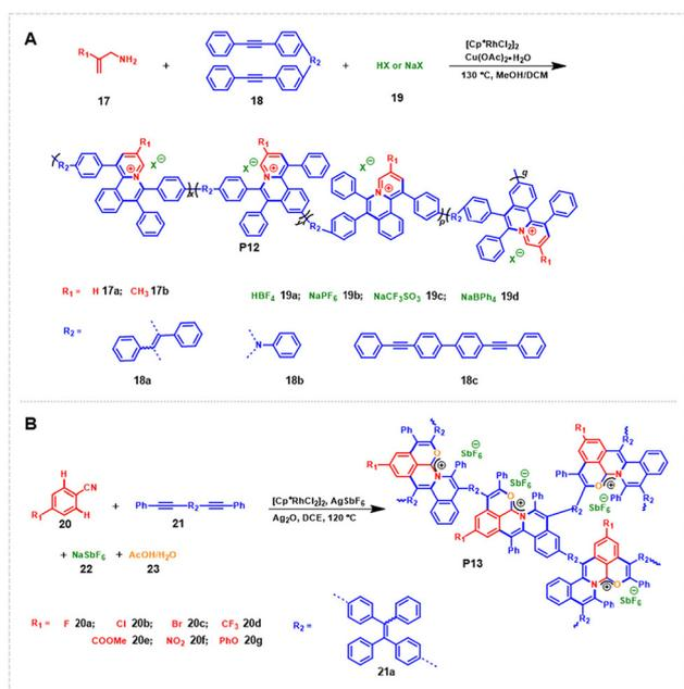
**Fig. 4** (A and B) Alkyne-based multicomponent polymerization methods. Reproduced with permission from (A) ref. 2 (Copyright 2019 American Chemical Society) and (B) ref. 18 (Copyright 2021 Wiley-VCH GmbH), respectively.
