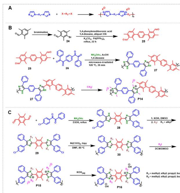
**Fig. 5** (A) The synthetic method of non-conjugated MCPs with imidazolium-salts. (B and C) The synthetic routes of imidazolium-containing CMCPs via the post-modification reaction. Reproduced with permission from (B) ref. 55 (Copyright 2017 American Chemical Society) and (C) ref. 56 (Copyright 2019 Springer Nature), respectively.
