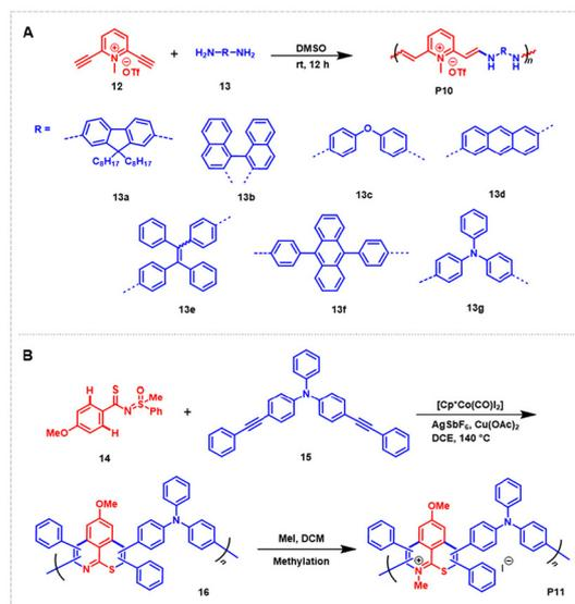
**Fig. 3** (A and B) Alkyne-based two-component polymerization methods. Reproduced with permission from (A) ref. 51 (Copyright 2024 ChemRxiv) and (B) ref. 52 (Copyright 2024 American Chemical Society), respectively.
