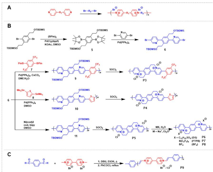
**Fig. 2** (A) The common method used for the synthesis of non-conjugated MCPs. (B and C) Synthesis of pyridinium-containing CMCPs *via* (B) nucleophilic substitution reactions and (C) aldol-type polycondensations. Adapted with permission from (B) ref. 48 (Copyright 2009 American Chemical Society), ref. 49 (Copyright 2014 Wiley-VCH GmbH), and (C) ref. 50 (Copyright 1989 Wiley-VCH), respectively.
