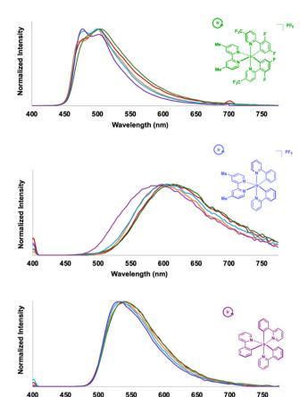
Fig. 1 Emission spectral overlays obtained for IrCat1 (top), IrCat2 (middle) and IrCat3 (bottom) in toluene, THF, DCM, MeCN, and DMSO. IrCat1 was excited at 350 nm while IrCat2 and IrCat3 were excited at 400 nm.
