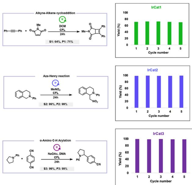
**Fig. 3** Recyclability of IrCat1 (top), IrCat2 (middle) and IrCat3 (bottom) in the alkyne–alkene cycloaddition, aza-Henry, and C–H arylation reactions, respectively. After reaction, the respective IrCat is recycled from the reaction mixture through multiple reprecipitations into methanol, followed by centrifugation, drying, and reuse in a fresh reaction.
