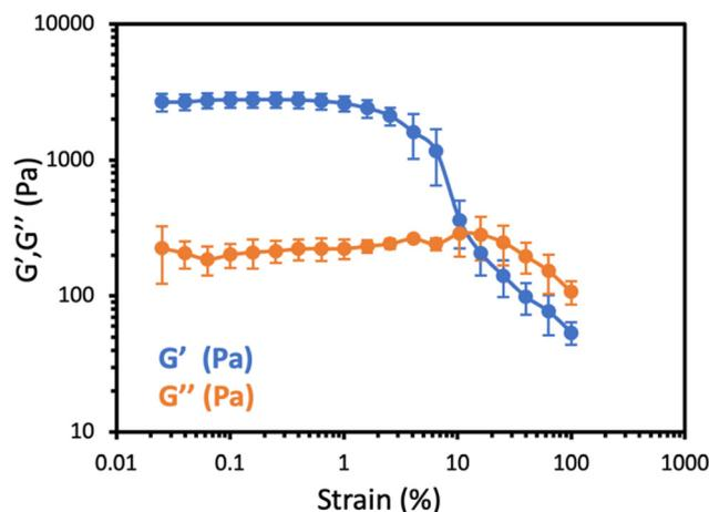
Fig. 2 Amplitude sweep test of the hydrogels obtained from 2:1 DBA-C6 $\times$ 2 (10 mg mL $^{-1}$ ) and TBA (5 mg mL $^{-1}$ ), at a constant frequency of 1 Hz.
