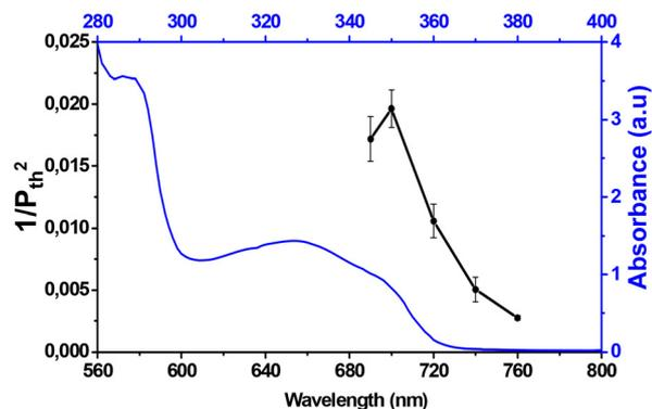
**Fig. 3** UV-visible absorbance spectra of alkoxyamine **5** in *tert*-butyl benzene solution ( $1.0 \times 10^{-4}$  M) (blue curve) and two-photon polymerization action spectra for PETA with 2 wt% alkoxyamine **5** (black line).
