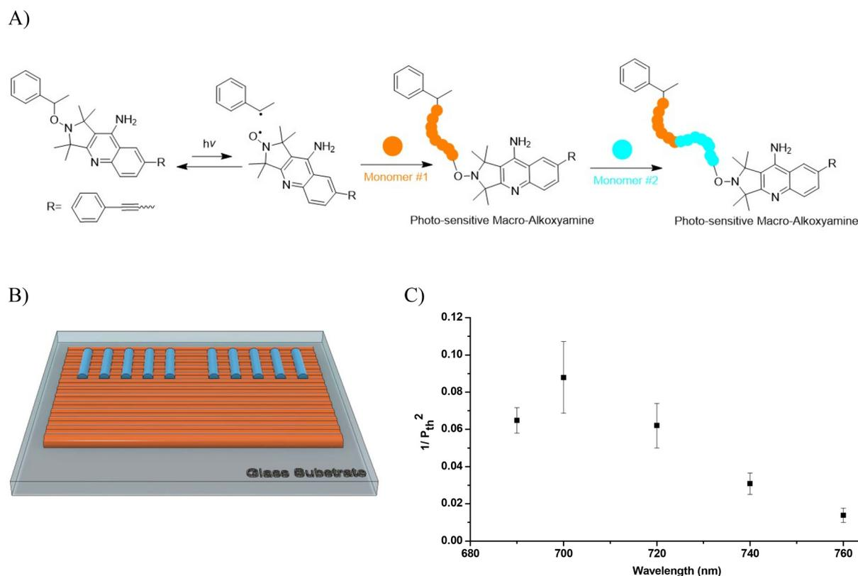
**Fig. 4** (A) Schematic presentation of the NMP2 two-photon stereolithography fabrication and surface functionalization processes. (B) Schematic presentation of written lines on the first layer and (C) two-photon re-polymerization action spectrum for TMPTA without addition of external photoinitiator at a wavelength range from 690 to 760 nm, under  $\text{N}_2$ .
