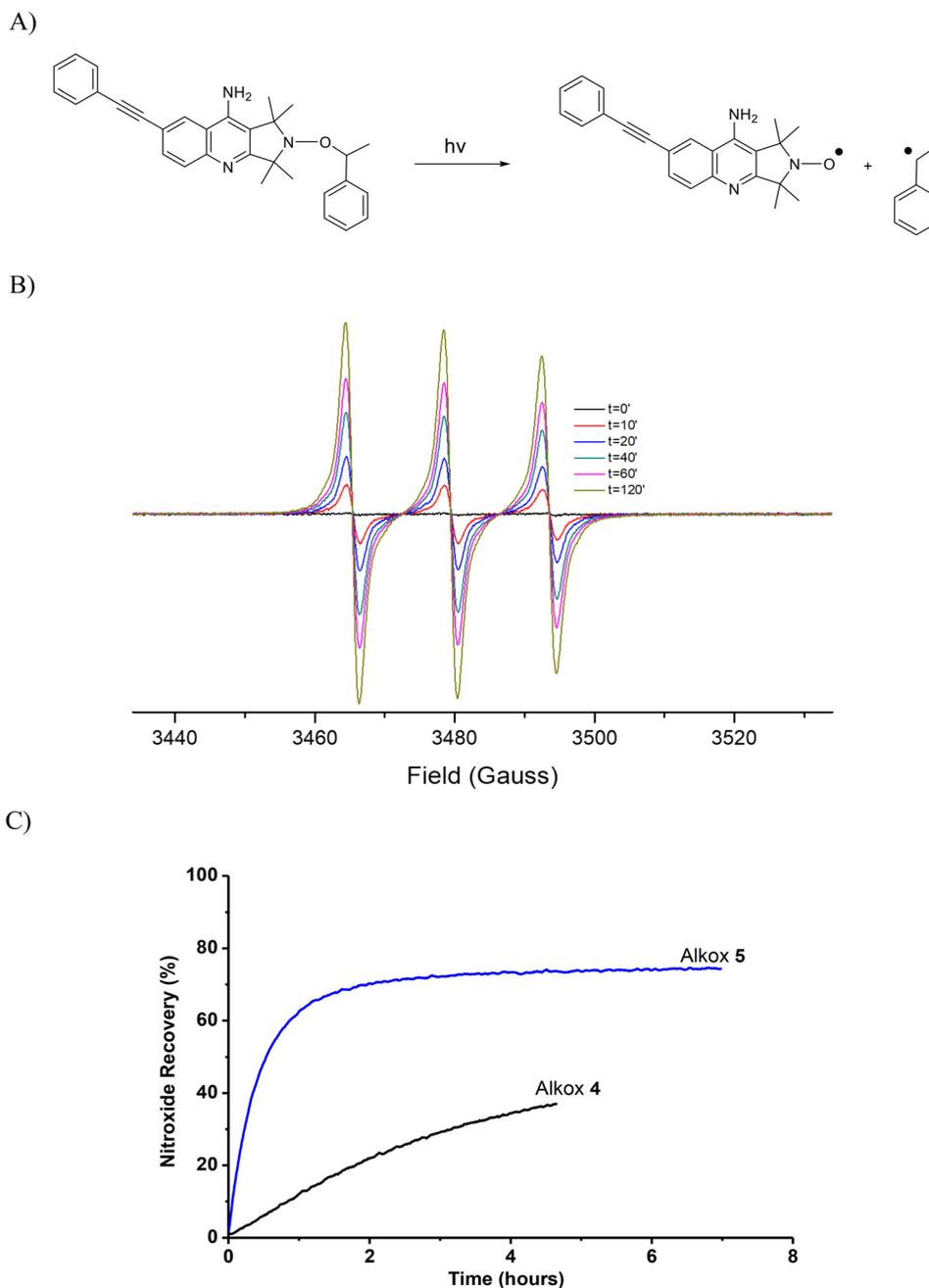
**Fig. 2** (A) Schematic photodissociation reaction of photosensitive alkoxyamine 5. (B) Evolution of the EPR spectrum of D- $\pi$ -A-based alkoxyamines 5 during the first 140 minutes of irradiation (C) nitroxide recoveries obtained for bromo alkoxyamine 4 and D- $\pi$ -A-based alkoxyamine 5 under UV irradiation using LC8 lamp at 10% of power (emission spectrum of this lamp in ESI, Fig. S8†).
