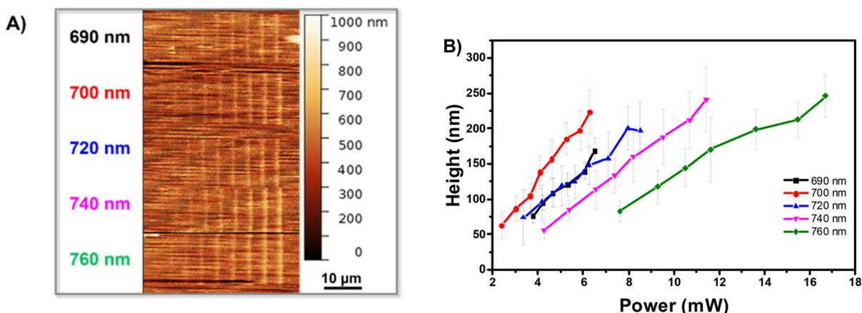
**Fig. 5** (A) AFM image of the two-photon re-polymerization of a series of lines on the surface of a first square fabricated at 15.6 mW and 740 nm at 690 nm, 700 nm, 720 nm, 740 nm, and 760 nm, exposure time = 10 ms with increasing the laser power (left to right) and (B) the evolution of the heights of written lines at different laser powers and wavelengths on the surface's bottom layer in the surface modification step.
