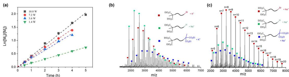
Fig. 3 (a) Plots of natural log of monomer conversion as a function of time for polymerization of **[M1]/[DBMM]/[PC1]** = 500/10/1 performed in PhCl (0.5 M), at  $\sim 30$  °C, with 1.4–10.8 W white LED irradiation. MALDI-TOF MS spectra of low-MW **PM1** synthesized with (b) 10.5 W and (c) 1.4 W white LED irradiation.
