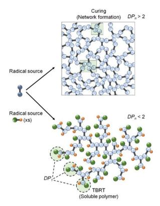
Fig. 1 Comparison of curing and network formation through the polymerisation of a multi-vinyl monomer and the creation of a soluble branched polymer by transfer-dominated branching telomerisation.
