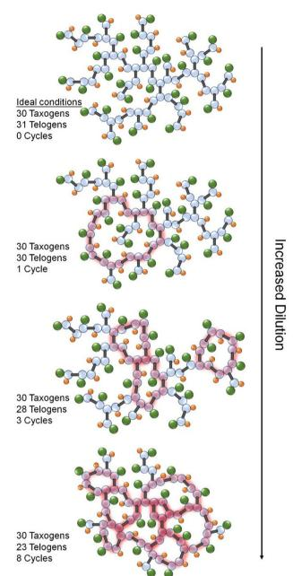
Fig. 2 Formation of branched polymers by TBRT containing increasing numbers of cycles if reactions are conducted at higher dilution. The number of telogens within the recovered polymer structure decreases with cycle formation.
