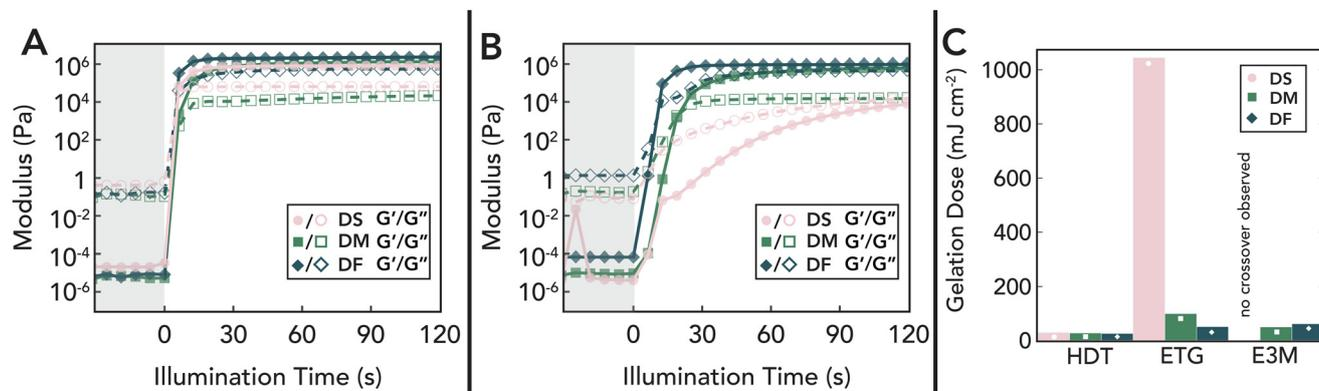
**Fig. 7** (A) Photorheology traces that depict rapid increases in modulus and crossover between storage and loss modulus during gelation in resins with HDT. (B) Photorheology shows the importance of the chain-growth mechanism on gelation kinetics in resins with EBTG. (C) Photo-dose for gelation obtained by the product of crossover time and light intensity for resins of different dithiols.
