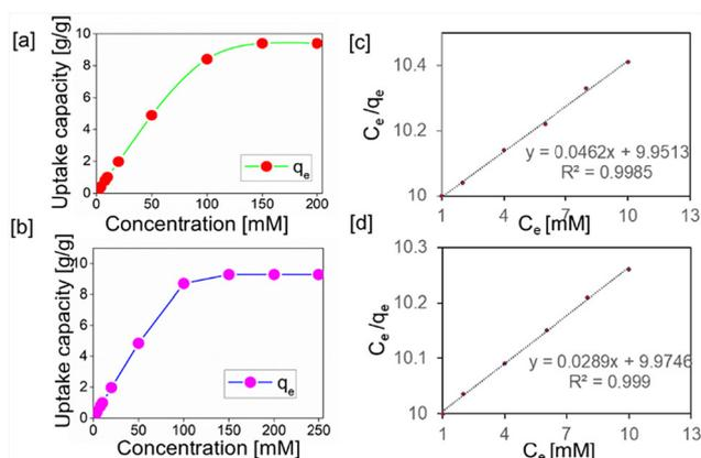
Fig. 5 Isotherm analyses of [a] **gn-ipop-cl(MC)** and [b] **gn-ipop-cl(ST)**. Langmuir adsorption model for [c] **gn-ipop-cl(MC)** and [d] **gn-ipop-cl(ST)**.
