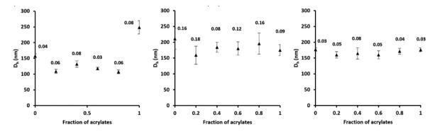
Fig. 2 Evolution of the hydrodynamic diameter for latexes of styrene, acrylates (n-BuA/MMA 50/50) or a mixture of those (weight fraction), stabilised with 10% w/w of (left) BRC<sub>1</sub>, (middle) BRC<sub>2</sub>, (right) BRC<sub>3</sub>. Numbers above the data point represent the PDI of these measurements.
