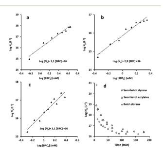
**Fig. 3** Evolution of  $N_{\rm p}$  while varying the concentration of BRC<sub>1</sub> (a), BRC<sub>2</sub> (b), BRC<sub>3</sub> (c). Evolution of  $N_{\rm p}$  during semi-batch polymerization of styrene, semi-batch polymerization of n-BuA/MMA (50/50 v/v) and batch polymerization of styrene (d).
