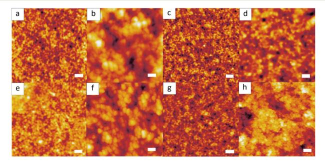
Fig. 1 AFM images of films of BRC at pH = 9.5 (a, c, e and g) and pH =  $pK_a$  (b, d, f and h) with BRC<sub>1</sub> (a and b) BRC<sub>3</sub> (c and d) BRC<sub>4</sub> (e and f) BRC<sub>5</sub> (g and h). Scale bar is 200 nm.
