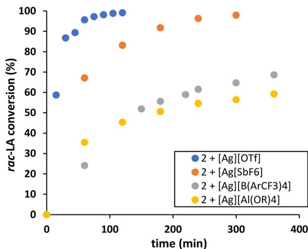
**Fig. 3** *rac*-LA conversion versus time for polymerisation initiated by **2** in the presence of different silver salts AgX (conditions: [*rac*-LA]<sub>0</sub> = 1 M, DCM, [2]/[AgX]/[*rac*-LA]<sub>0</sub> = 1/1/100).
