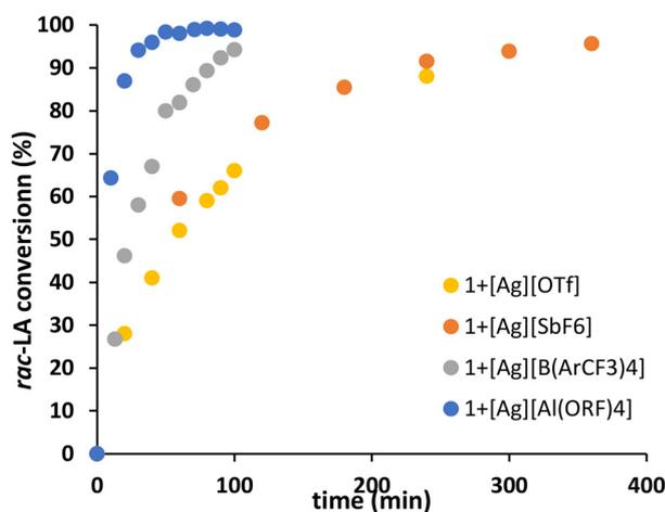
**Fig. 2** *rac*-LA conversion versus time for polymerisation initiated by **1** in the presence of different silver salts AgX (conditions: [*rac*-LA]<sub>0</sub> = 1 M, DCM, [1]/[AgX]/[*rac*-LA]<sub>0</sub> = 1/1/100).
