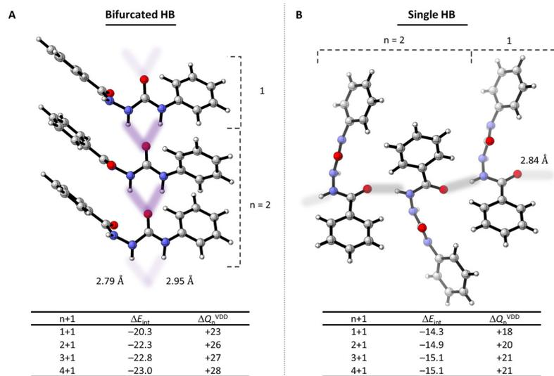
**Fig. 3** Hydrogen-bonding patterns found in the crystal structure of PhASCPH depicting bifurcated (A) and single (B) hydrogen bonds. Hydrogen bond lengths  $r_{\text{O-N}}$  (in Å), interaction energies  $\Delta E_{\text{int}}$  (in kcal mol<sup>-1</sup>), and charge transfer values  $\Delta Q_n^{\text{VDD}}$  (in milli-electrons) are shown, computed at a ZORA-BLYP-D3(BJ)/TZ2P level of theory. The chain elongation direction is from bottom to top (A) and from left to right (B).
