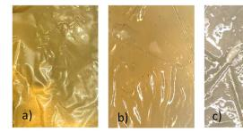
Fig. 11 Photographs of three different blend membranes with Ter-Phos (a) p-PSUa: Ter-Phos, 1:1; (b) p-PSUb: Ter-Phos, 1:1; (c) p-PSUs: Ter-Phos, 1:1.
