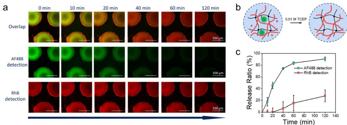
**Fig. 6** (a) Time series of fluorescence microscopy images of HRP- and poly(NiPAAm-co-RhBA)-containing  $\mu$ HDs under TCEP reduction, with the scale bar of 500  $\mu$ m. (b) Schematic drawing of the release of HRP and of enzymatically synthesized poly(NiPAAm-co-RhBA) from  $\mu$ HDs by TCEP. (c) Release of HRP-AF488-PDA and of poly(NiPAAm-co-RhBA) by TCEP reduction as measured by the relative reduction in fluorescence intensity of the microscopy images shown in (a).
