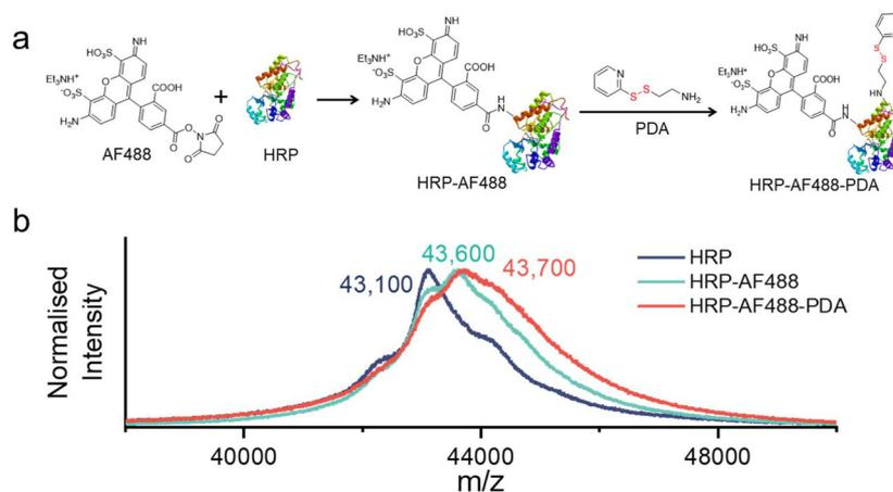
**Fig. 3** (a) Reaction scheme of the modification of HRP with the fluorescent dye AF488 and disulphide bonds (PDA). (b) MALDI-TOF MS spectra in the  $[M + X]^+$  ( $X$ : Na or H) range of HRP, HRP-AF488, and HRP-AF488-PDA.
