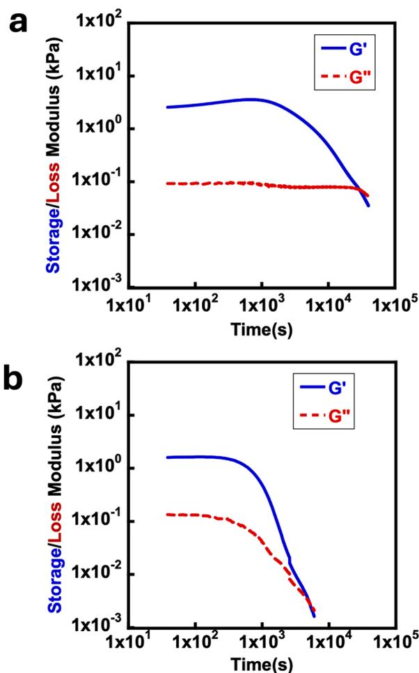
Fig. 4 Typical rheology time sweeps at 15 °C using a frequency of 10 rad s<sup>-1</sup> with 1 M EDC for deprotected (a) poly(O<sub>N</sub>B<sub>M</sub><sub>15</sub>-DMAM<sub>81</sub>) and (b) poly(O<sub>N</sub>B<sub>M</sub><sub>15</sub>-DMAM<sub>122</sub>).
