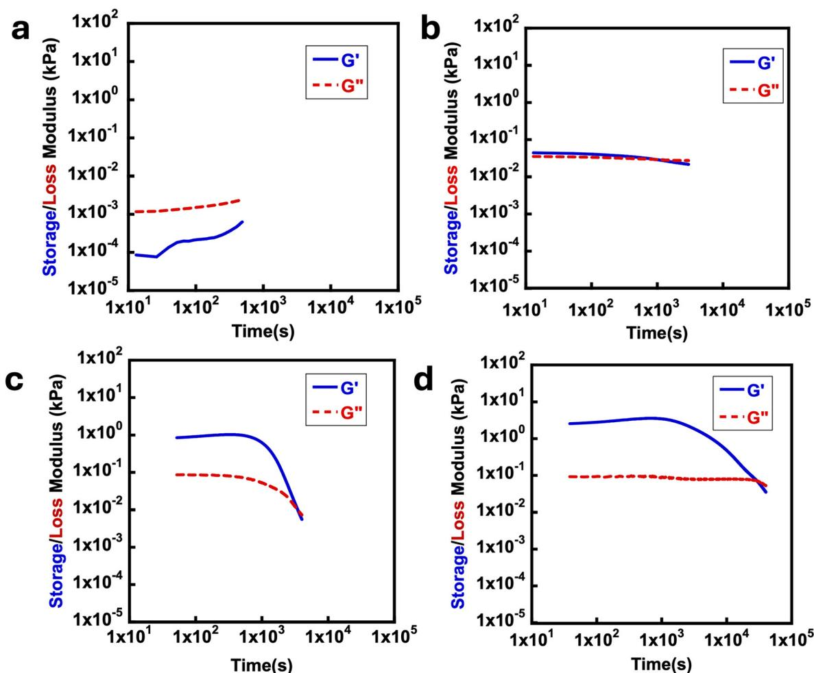
Fig. 2 Typical rheology time sweeps at  $15 \text{ }^\circ\text{C}$  using a frequency of  $10 \text{ rad s}^{-1}$  for poly(ONBM<sub>15</sub>-DMAM<sub>81</sub>) exposed to  $360 \text{ nm}$  UV for (a) 8 h then 1 M EDC, (b) 8 h then 2 M EDC (c) 16 h then 1 M EDC and (d) 24 h then 1 M EDC.
