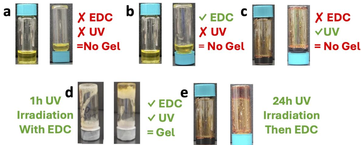
**Fig. 1** Inverted vial tests for (a) protected poly(ONBM<sub>15</sub>-DMAM<sub>81</sub>) without the addition of EDC, (b) protected poly(ONBM<sub>15</sub>-DMAM<sub>81</sub>) with EDC added, (c) deprotected poly(ONBM<sub>15</sub>-DMAM<sub>81</sub>) without EDC, (d) protected poly(ONBM<sub>15</sub>-DMAM<sub>81</sub>) with EDC added then exposed to 360 nm UV for 1 h, and (e) deprotected poly(ONBM<sub>15</sub>-DMAM<sub>81</sub>) with EDC added.
