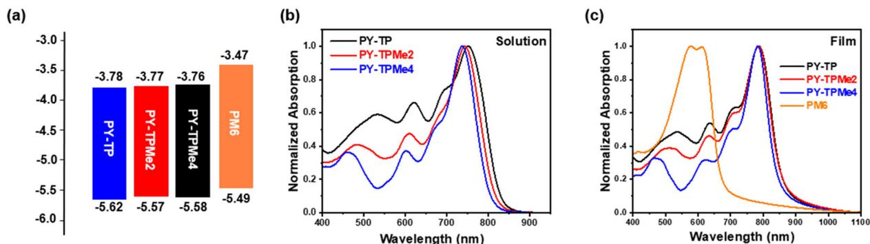
**Fig. 2** (a) The energy level diagrams of PM6, PY-TP, PY-TPMe2 and PY-TPMe4. (b) Normalized absorption spectra of PY-TP, PY-TPMe2 and PY-TPMe4 in solution. (c) Normalized absorption spectra of PM6, PY-TP, PY-TPMe2 and PY-TPMe4 in films.
