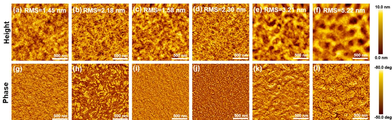
Fig. 4 (a–f) AFM height images of (a) as-cast PM6:PY-TP, (b) optimized PM6:PY-TP, (c) as-cast PM6:PY-TPMe2, (d) optimized PM6:PY-TPMe2, (e) as-cast PM6:PY-TPMe4 and (f) optimized PM6:PY-TPMe4. (g–l) AFM phase images of (g) as-cast PM6:PY-TP, (h) optimized PM6:PY-TP, (i) as-cast PM6:PY-TPMe2, (j) optimized PM6:PY-TPMe2, (k) as-cast PM6:PY-TPMe4 and (l) optimized PM6:PY-TPMe4.
