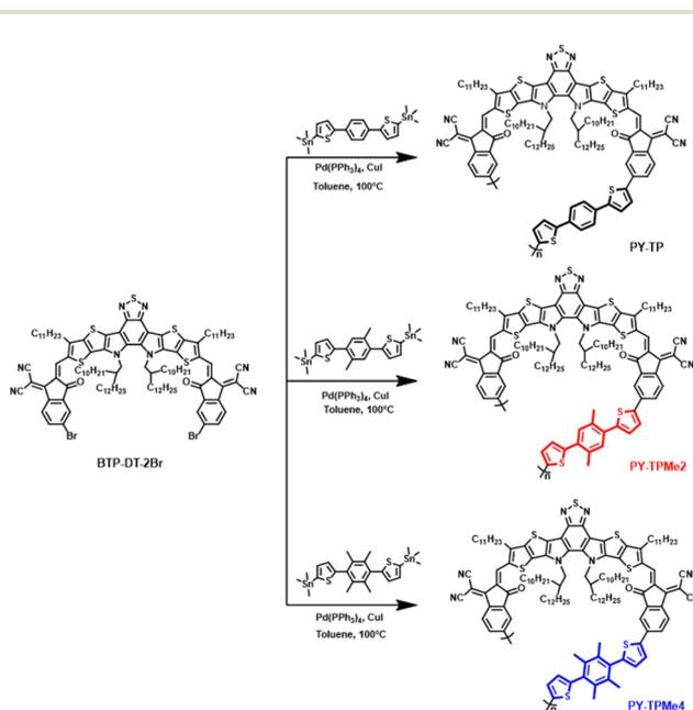
Scheme 1 Synthesis routes of PY-TP, PY-TPMe<sub>2</sub> and PY-TPMe<sub>4</sub>.
