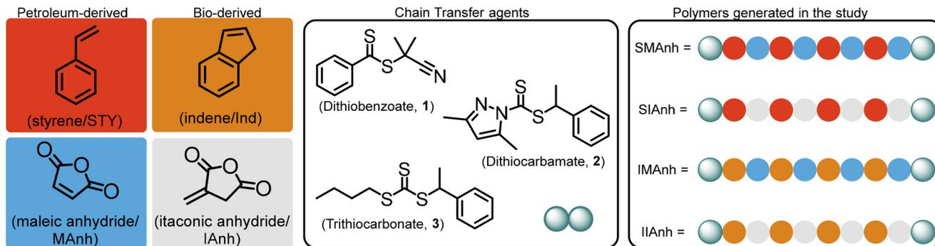
**Fig. 1** Copolymers synthesized using styrene (STY), indene (Ind), maleic anhydride (MAAnh), and itaconic anhydride (IAAnh). poly(styrene-*alt*-maleic anhydride) (SMAAnh), poly(styrene-*alt*-itaconic anhydride) (SIAnh), poly(indene-*alt*-itaconic anhydride) (IIAnh), poly(indene-*alt*-maleic anhydride) (IMAnh).
