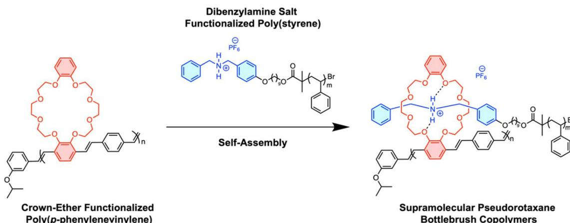
**Scheme 2** Synthesis of supramolecular bottlebrush copolymers based on host–guest interactions between crown-ether functionalized poly(*p*-phenylenevinylene) and dibenzyl amine end-functionalized poly(styrene).
