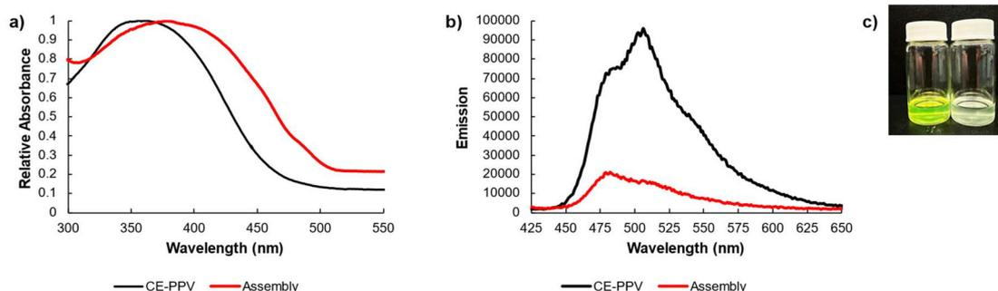
Fig. 4 (a) Absorbance spectra and (b) emission spectra of homopolymer CE-PPV (**13b**) (black) and the supramolecular bottlebrush CE-PPV-PS-DBA<sup>+</sup> (red). (c) The CE-PPV has strong fluorescence (left) and the bottlebrush has quenched fluorescence (right).
