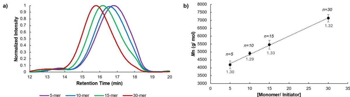
Fig. 1 (a) Molecular weight distribution of polymers **13a–d** (GPC in THF). (b) Dependence of  $M_n$  as measured by GPC of polymers **13a–d** on the  $[M]/[I]$  ratio. Here, **13a**,  $n = 5$ , **13b**,  $n = 10$ , **13c**,  $n = 15$ , and **13d**,  $n = 30$ . Dispersity values of the respective polymers are denoted in the plot.
