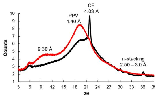
Fig. 5 WAXS diffractograms corresponding to homopolymer CE-PPV (**13b**) (black) and the supramolecular bottlebrush CE-PPV-PS-DBA<sup>+</sup> (red).
