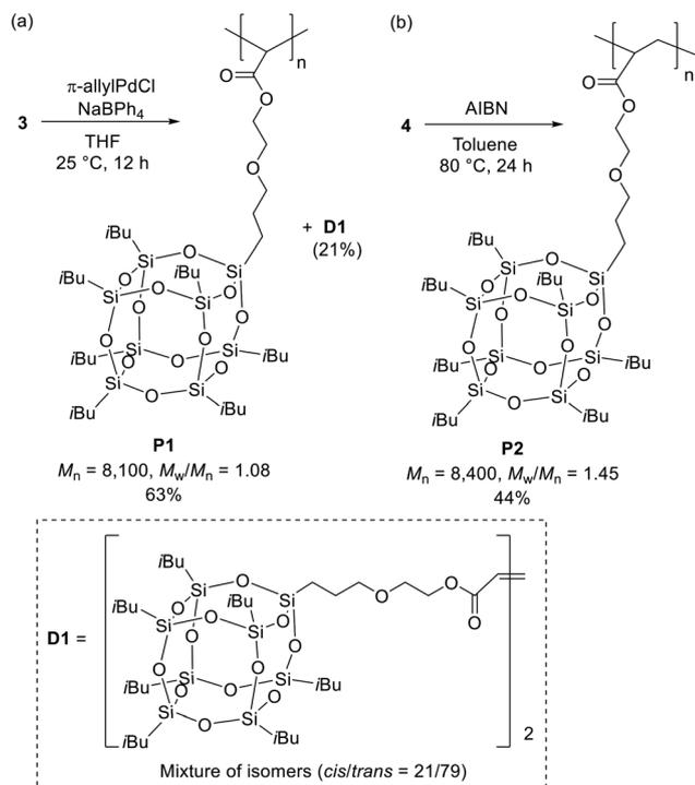
**Scheme 2** Syntheses of (a) polymer **P1** and dimer **D1**, and (b) polymer **P2**.
