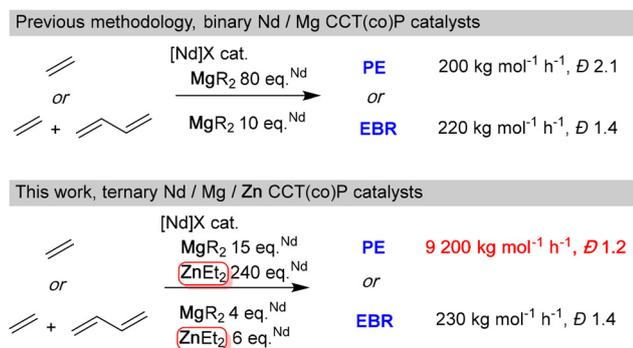
**Scheme 1** Implementation of the CCTP of ethylene and CCTcoP of ethylene and butadiene mediated by binary or ternary Nd-based catalysts. [Nd] corresponds to the metal center and its ligands (Me<sub>2</sub>Si(C<sub>13</sub>H<sub>8</sub>)<sub>2</sub>), [Nd]X =  $\{[(\text{Me}_2\text{Si}(\text{C}_{13}\text{H}_8)_2)\text{Nd}(\mu\text{-BH}_4)[(\mu\text{-BH}_4)\text{Li}(\text{THF})]]_2\}$ .
