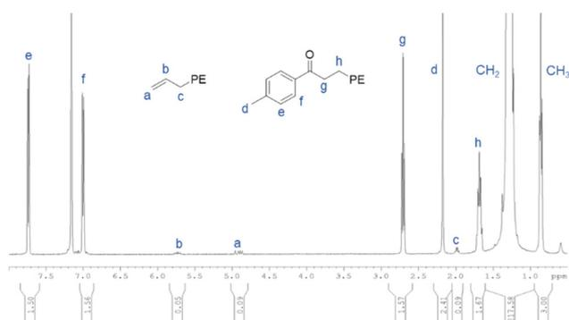
**Fig. 2** <sup>1</sup>H NMR spectrum of the *p*-methylphenone-PE obtained with the ternary catalytic system 1/MesMgBr/ZnEt<sub>2</sub> after deactivation with *p*-toluoyl chloride (run 16, Table 5).
