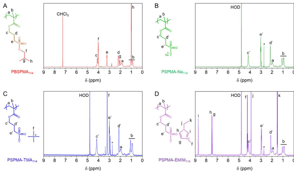
**Fig. 1** Comparative  $^1\text{H}$  NMR spectra (400 MHz) of (A) protected  $\text{PBSPMA}_{114}$  and polyelectrolytes featuring various counterions, including: (B)  $\text{PSPMA-Na}_{114}$ , (C)  $\text{PSPMA-TMA}_{114}$  and (D)  $\text{PSPMA-EMIM}_{114}$ .
