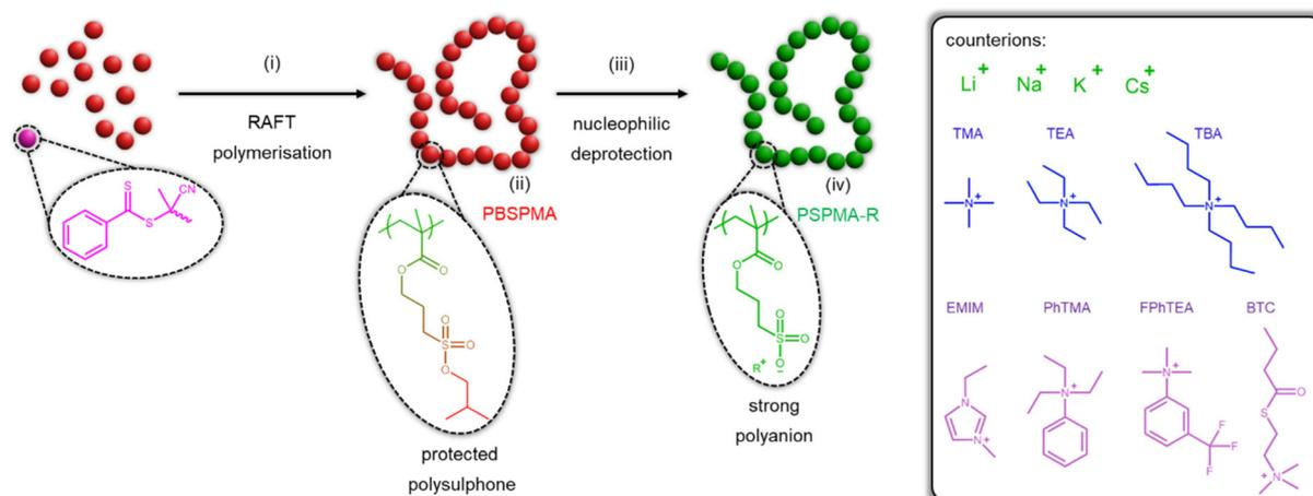
**Scheme 1** Tailoring the nature of the polyelectrolyte counterion through nucleophilic deprotection. (i) Controlled radical polymerisation is used to produce (ii) a protected poly(3-isobutoxysulphopropyl methacrylate) homopolymer. (iii) Subsequent nucleophilic deprotections using iodide-based salts are performed to remove the protective groups and yield (iv) a range of strong poly(sulphopropyl methacrylate) polyanions featuring various inorganic and organic counterions.
