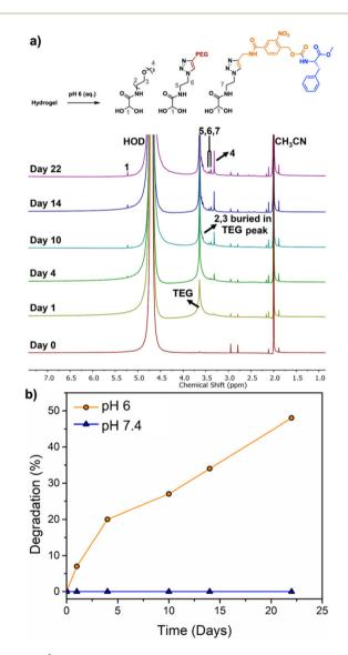
Fig. 5 (a) <sup>1</sup>H NMR spectra of the Phe-oNB-TEG-N<sub>3</sub>-30-PGAm hydrogel in deuterated PBS (pH 6) containing 1% CH<sub>3</sub>CN; (b) percent hydrogel degradation versus time at pH 6 and 7.4 as determined based on the integral of peak 4 compared to the CH<sub>3</sub>CN internal standard peak.
