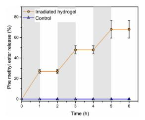
Fig. 4 Release of Phe methyl ester from irradiated Phe-oNB-TEG-N $_3$ -30-PGAm hydrogel immersed in PBS at 37 °C. Periods of irradiation with light are indicated by grey shading. Data are presented as the mean  $\pm$  standard deviation (n=3), except for the control where no error bars are included as no amine was detected.
