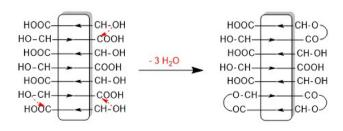
Scheme 1 SSP via formation of loops on the surface of crystallites
