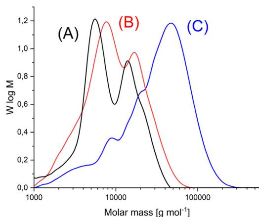
**Fig. 5** SEC mass distribution curves of (A) HO-PLA-25, (B) annealed with SnOct<sub>2</sub>, at 140 °C for 14 d (2A, Table 3), (C) annealed with SnOct<sub>2</sub> at 160 °C for 6 d (2B, Table 4).
