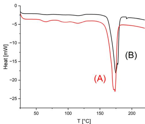
Fig. 7 DSC traces (1<sup>st</sup> heating) of HO-PLA-12 annealed at 140 °C for 14 d: (A) with  $\text{SnCl}_2$  (3, Table 1), (B) with TSA (4, Table 2).
