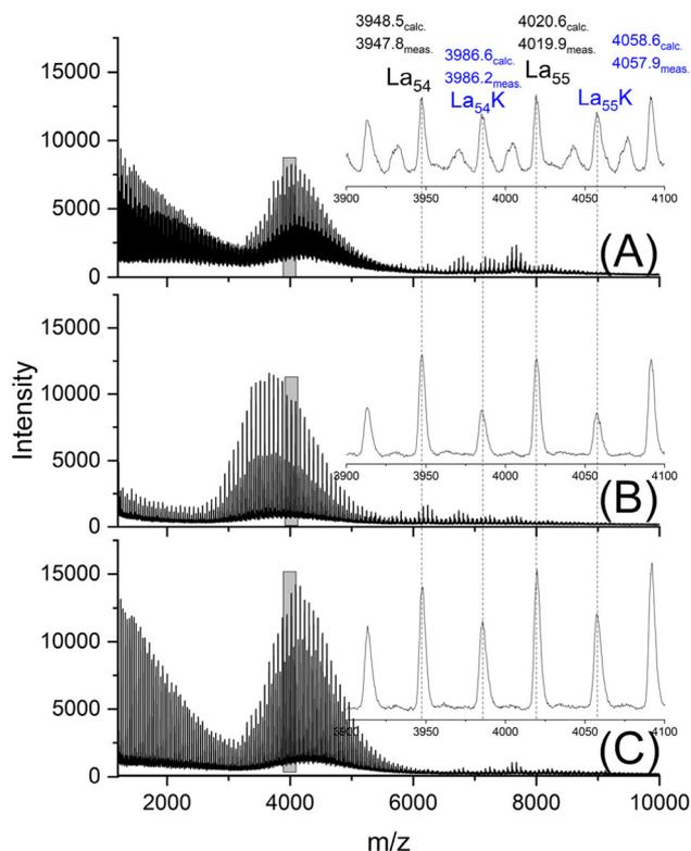
**Fig. 6** MALDI-TOF mass spectra of HO-PLA-50 annealed at 140 °C for 14 d; (A) with SnOct<sub>2</sub> (2A, Table 4), (B) with SnCl<sub>2</sub> (3A, Table 4), (C) with TSA (4A, Table 4).
