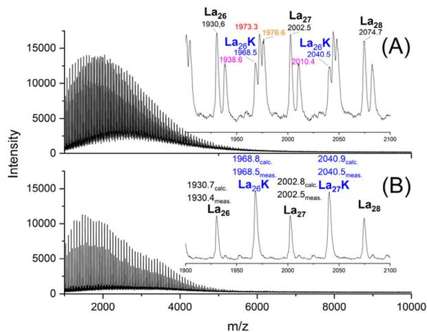
**Fig. 1** MALDI TOF mass spectra PLAs prepared by polycondensation of LA: (A) catalyzed with  $\text{SnCl}_2$  after 6 d at 140 °C (1B, Table 1), (B) catalyzed with TSA after 6 d at 140 °C (2B, Table 1).
