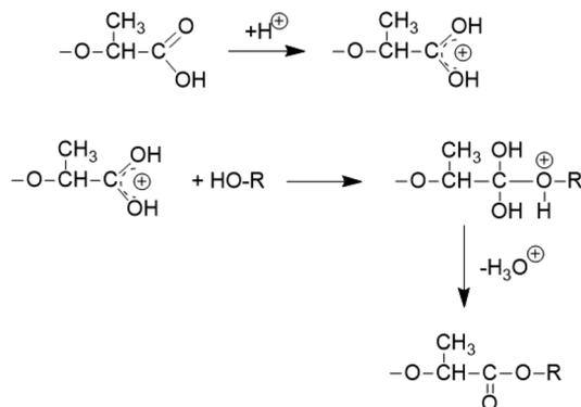
**Scheme 4** Proton (TSA)-catalyzed esterification of lactic acid units.
