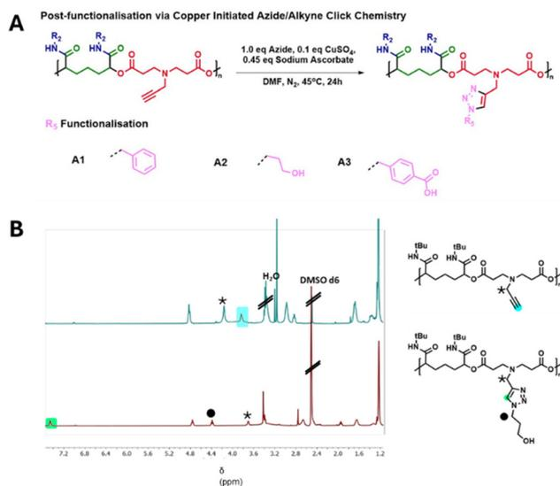
**Fig. 5** (A) Synthesis of post-modified Passerini derived polymers via copper-initiated azide/alkyne click. (B)  $^1\text{H}$  NMR spectra of polymer D2-I1 (top) and the product D2-I1-A2 (bottom) following functionalisation via copper/click chemistry.
