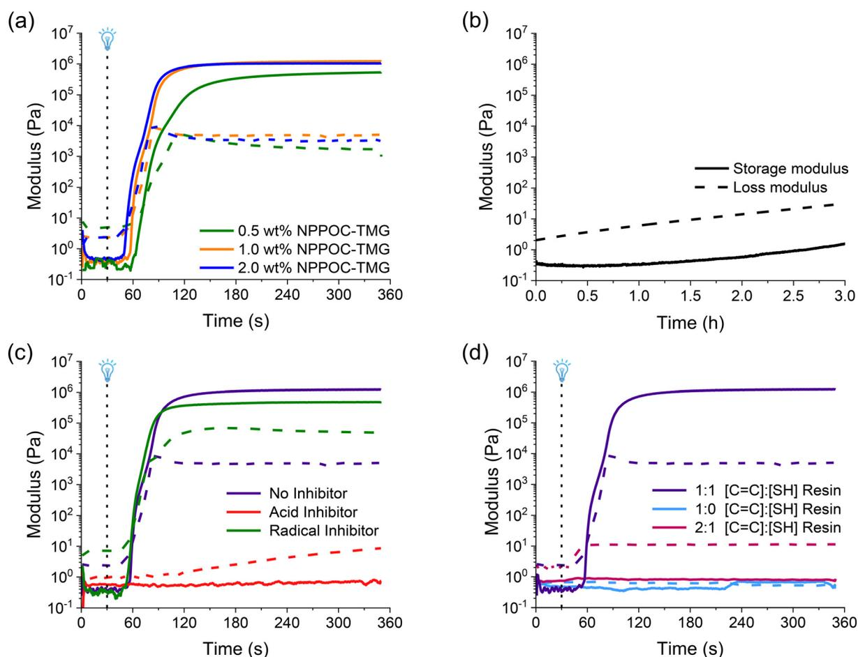
**Fig. 2** Rheology of thiol-Michael resins; dashed lines are  $G''$  and solid lines are  $G'$ . Rheological conditions for photorheology: 1 Hz, 1% strain, light on at 30 s. (a) UV curing experiment showing the effect of NPPOC-TMG concentration. (b) Dark stability of the resin (5 Pa strain amplitude, no light, 3 h). (c) UV curing of resins with radical inhibitor or organic acid. (d) UV curing comparing resins without trithiol monomer and substoichiometric thiol content.
