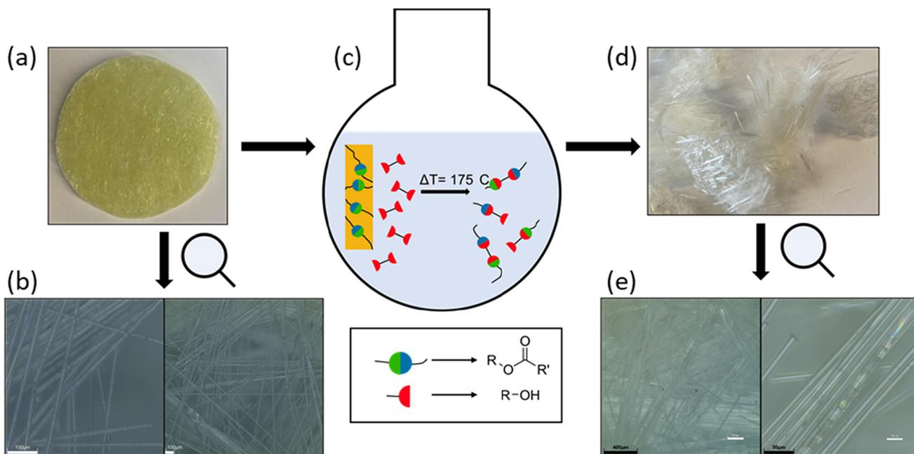
**Fig. 5** (a) Frontally cured composite of glass fibres and SH20; (b) microscopy images of the virgin glass fibres at 140-fold magnification and at 500-fold magnification; (c) scheme of depolymerization in ethylene glycol; (d) recovered glass fibres; (e) microscopy images of recovered glass fibres at 140-fold magnification and at 500-fold magnification.
