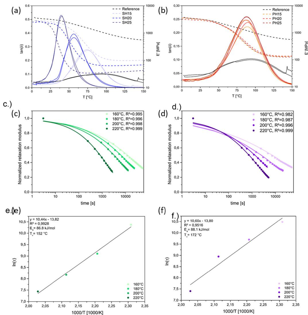
**Fig. 3** Mechanical properties; DMA-curves of frontally cured samples (a) with varying thiol and (b) phosphate content; KWW modelled stress-relaxation measurements (c) of SH20 and (d) PH20 obtained at varying temperature; the Arrhenius plot of (e) SH20 and (f) PH20 with calculated  $T_v$  and  $E_a$ .
