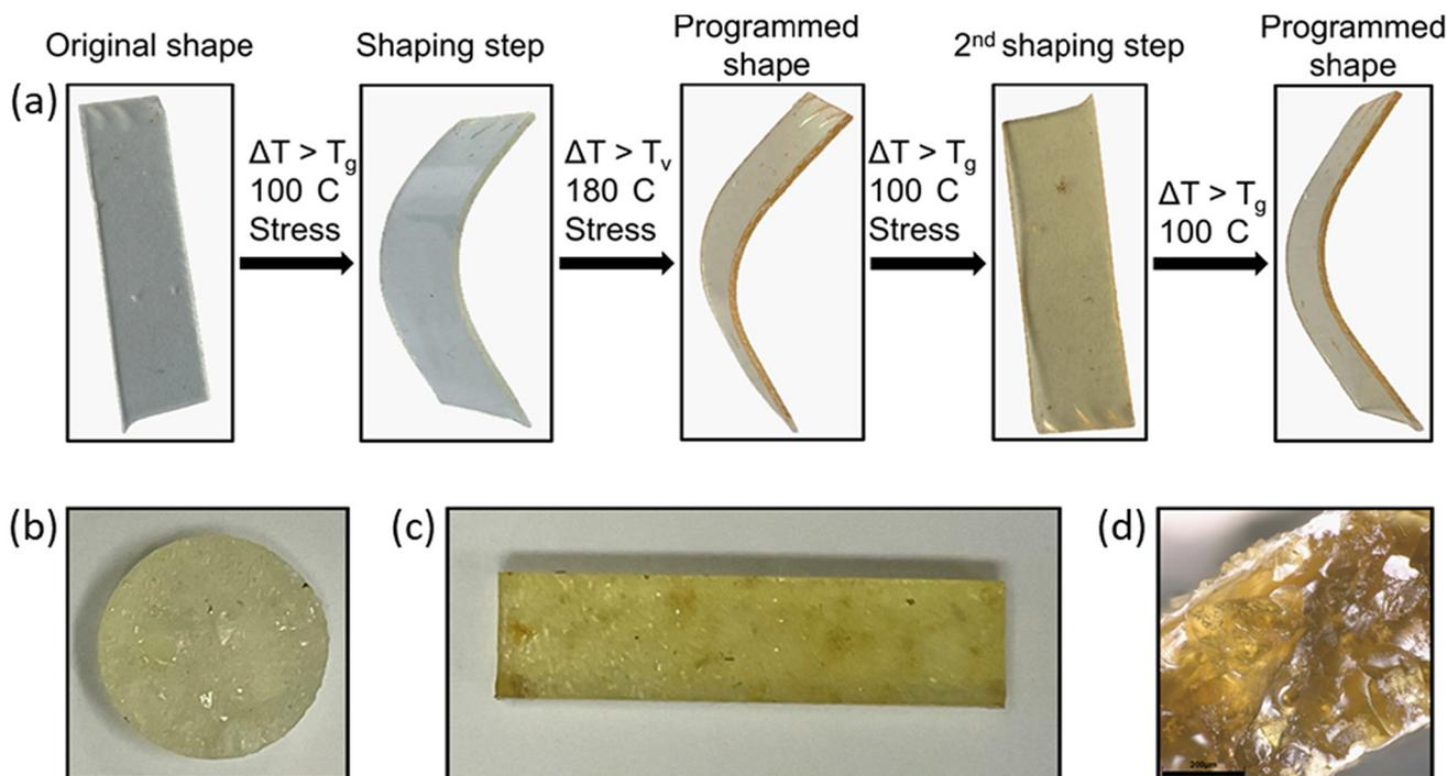
**Fig. 4** (a) Reshaping of frontally cured SH20 over  $T_g$  and reprogramming over  $T_v$  and subsequent 2<sup>nd</sup> reshaping over  $T_g$ ; (b) 8 mm  $\varnothing$  sample made with the VCM device at 170 °C for 1 h; (c) sample made with the VCM device at 210 °C for 1 h; (d) microscopy cross-section of the pressed sample.
