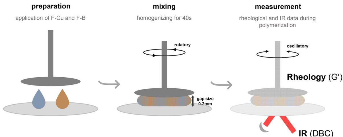
**Fig. 1** The work-flow of rheology/IR measurements is depicted, starting with preparation of the formulations containing the respective Cu and diborane and their application to the rheometer. Thereafter a mixing phase of 40 s in rotary mode ensures a homogeneous mixture of the 2K system. Subsequently, the rheological measurements records  $G'$  and  $G''$  in oscillatory mode and the NIR measurement starts simultaneously.
