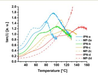
Fig. 3 Comparison of the DMTA measurements (temperature dependent  $\tan(\delta)$ -curves) of the model polymers MP-2a, MP-2c and MP-2d as well as the interpenetrating metallopolymer networks IPN-a to IPN-d.
