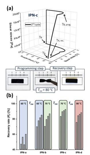
**Fig. 4** (a) 3D-TMA plot (2<sup>nd</sup> cycle) and photo-series of the manual shape-memory test for **IPN-c** and (b) comparison of the strain fixity and recovery rates of the IPNs determined *via* TMA over four cycles.
