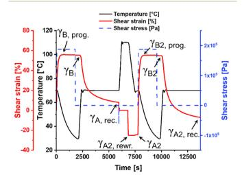
Fig. 5 2D-TMA plot (rewriting experiment) of IPN-c\*.
