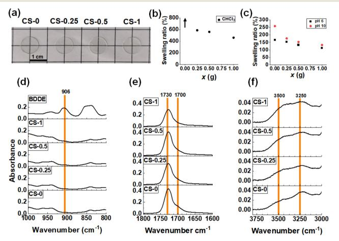
Fig. 2 (a) Photographs of each of the Stage I + II films (thickness = 0.5 mm). (b) The swelling ratios of the films in CHCl<sub>3</sub> after 5 days. The arrow shows that the CS-0 film, which swelled considerably, became too brittle to measure. (c) Swelling ratio of the films in water at pH 6 and 10. Expanded views of the FTIR spectra for the (d) epoxide region, (e) C=O region and (f) -OH region (see the text).
