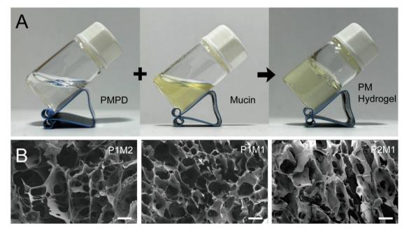
Fig. 3 (A) Formation of hydrogel via mixing the solutions of PMPD and mucin. (B) SEM images of P1M2, P1M1, and P2M1 hydrogels. Scale bar = 100 μm.
