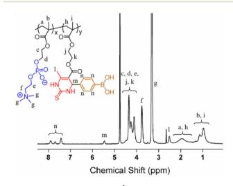
**Fig. 2** The chemical structure and <sup>1</sup>H NMR spectrum of zwitterionic PMPD copolymer.
