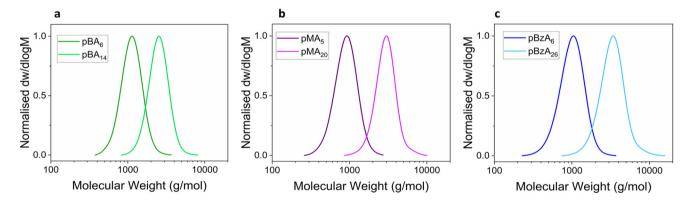
Fig. 3 SEC DRI traces of (a) N<sub>3</sub>pBA<sub>6</sub>, N<sub>3</sub>pBA<sub>14</sub> (b) N<sub>3</sub>pMA<sub>5</sub>, N<sub>3</sub>pMA<sub>20</sub> and (c) N<sub>3</sub>pBnA<sub>6</sub> and N<sub>3</sub>pBnA<sub>26</sub> in CHCl<sub>3</sub>. Molecular weights were calculated according to PMMA standards for a, b and pSt for c
