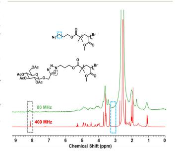
Fig. 5 <sup>1</sup>H-NMR spectra in DMSO of N<sub>3</sub>pMA<sub>5</sub> (0.18 M) using an 80 and a 400 MHz instrument after 42 min of the reaction with GlcAcPr in flow.
