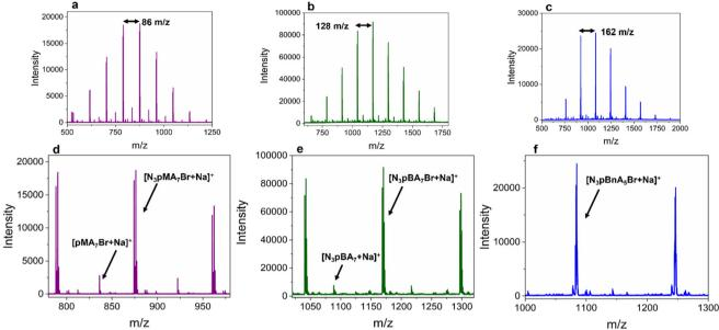
Fig. 4 MALDI TOF MS spectra of the three synthesised polyacrylates in THF using trans-2-[3-(4-tert-butylphenyl)-2-methyl-2-propyldene] malonitrile as a matrix. (a)  $N_3pMA_5$ , (b)  $N_3pBA_6$ , (c)  $N_3pBnA_6$ , (d) zoomed area for  $N_3pMA_5$ , (e) zoomed area for  $N_3pBnA_6$ , (f) zoomed area for  $N_3pBnA_6$ .
