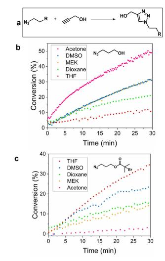
Fig. 1 (a) Reaction scheme of the studied "click" reaction. Conversions of the CuAAC reaction with propargyl alcohol in different solvents at 20 °C on a benchtop NMR at 80 MHz (b) with azidopropanol and (c) APBIB.
