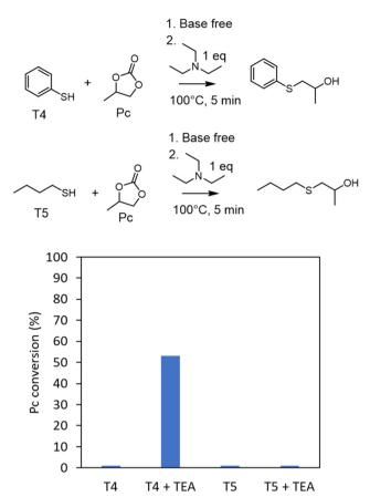
Fig. 2 Propylene carbonate (Pc) conversion when reacted with thiophenol (T4) or 1-butanethiol (T5) in the presence or absence of triethylamine (TEA) determined by 1-H NMR spectroscopy (see Fig. S1† for NMR spectra). Conditions: propylene carbonate (5 mmol), thiol (5 mmol), TEA (5 mmol), preheating of the components at 100 °C before mixing them, followed by reaction at 100 °C for 5 min in a closed vial.
