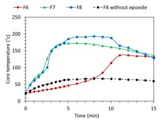
Fig. 5 Room temperature foaming using an epoxide additive for exotherms. Conditions: TMPTC, [5CC]: [epoxide]:  $[NH_{2 total}]$ : [SH] = 1:1:1.5:0.5
