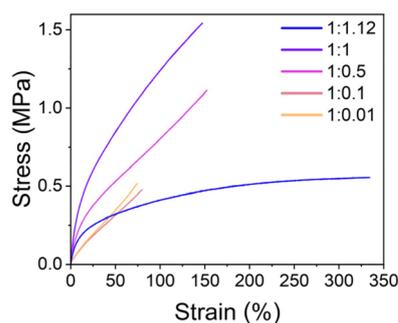
**Fig. 2** Representative curves for the tensile test of samples with different SP-Ep : ZnCl<sub>2</sub> (x : y) ratios.
