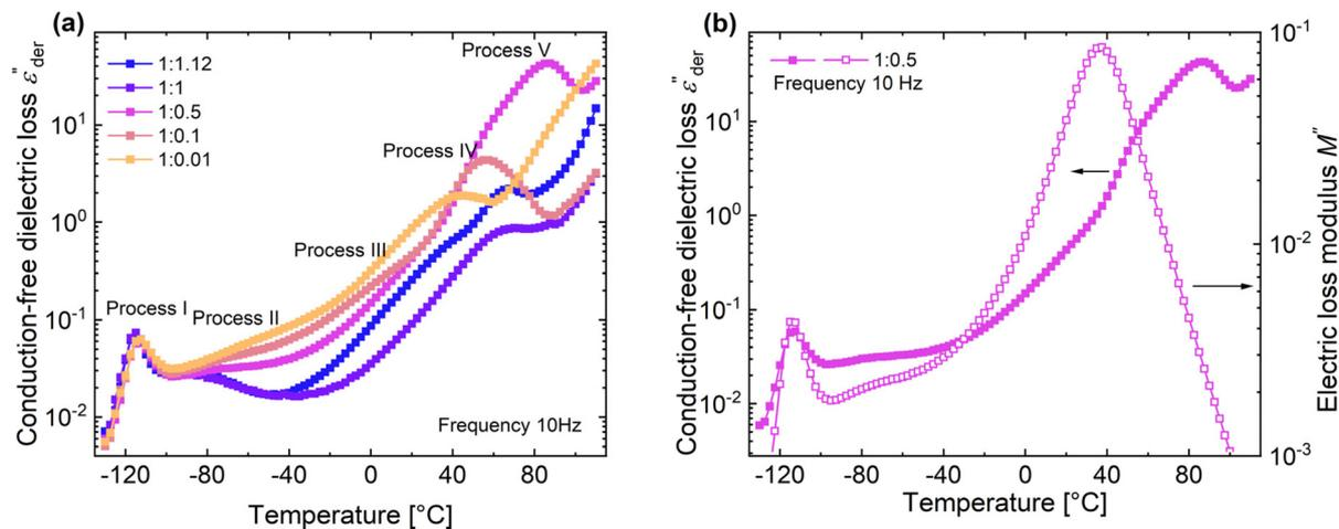
**Fig. 6** (a) D.C. conduction-free dielectric loss ( $\epsilon''_{\text{der}}$ ) curves of different SP-Ep:ZnCl<sub>2</sub> samples as a function of temperature at 10 Hz. (b)  $\epsilon''_{\text{der}}$  and dielectric loss modulus  $M''$  temperature of 1:0.5 and 1:0.1 samples as a function of temperature at 10 Hz.
