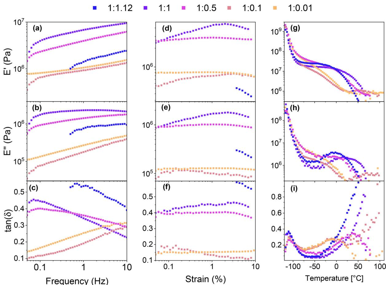
**Fig. 3** Dynamic mechanical analysis of different samples: the storage modulus, loss modulus, and  $\tan(\delta)$  in the frequency mode (a), (b), and (c); strain sweep (d), (e), and (f); and in dependence of the temperature (g), (h), and (i). All curves represent the average of at least three measurements.
