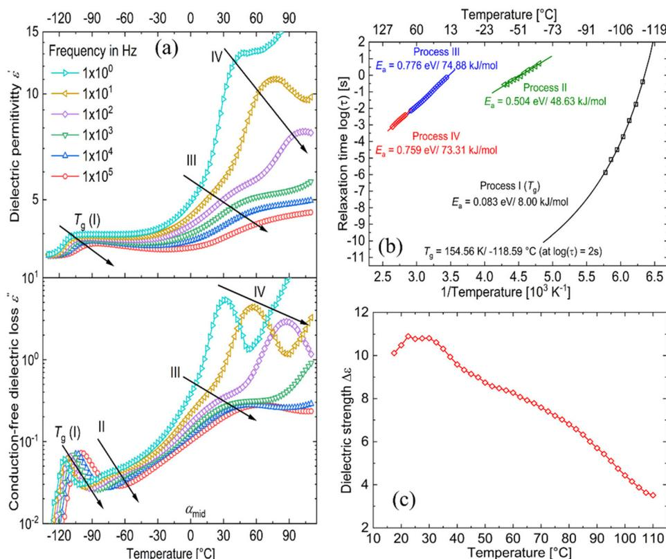
**Fig. 5** Dielectric analysis of a 1 : 0.1 SP-Ep : ZnCl<sub>2</sub> sample (a) real part of dielectric permittivity ( $\epsilon'$ ) and d.c. conduction-free dielectric loss ( $\epsilon''_{der}$ ) as a function of temperature at selected frequencies. (b) Arrhenius relaxation plot of all the observed relaxations. (c) Dielectric strength ( $\Delta\epsilon$ ) of the observed relaxations between 20 and 110 °C.
