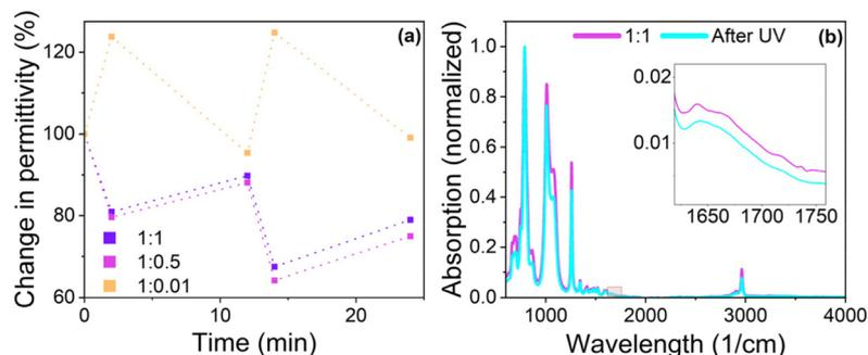
**Fig. 8** Relative change in permittivity at 1 kHz of sample 1 : 1, 1 : 0.5, and 1 : 0.01 after exposure to UV for 2 min followed by green light 10 min (2 cycles) (a). Absorption spectra of 1 : 0.5 before and after UV light (b).
