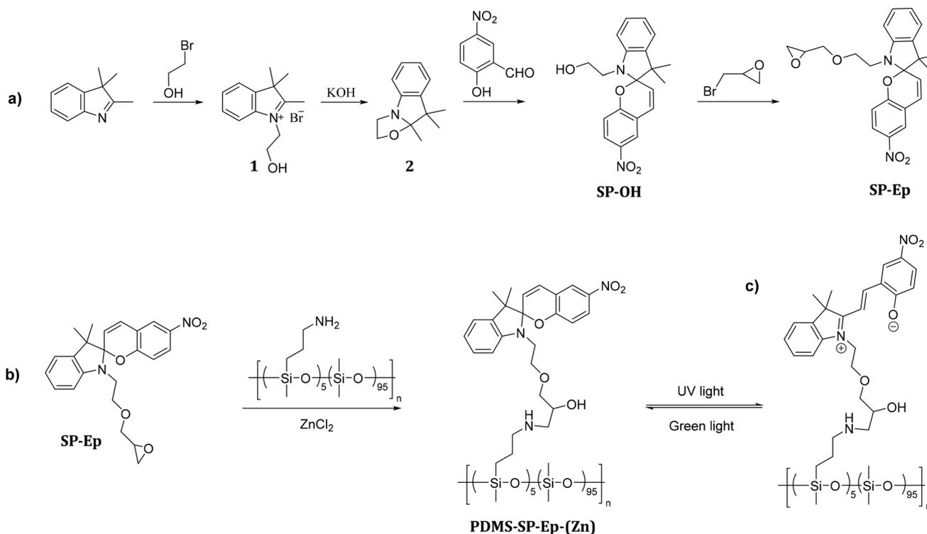
**Scheme 1** Synthetic pathway for the photoswitch SP-Ep (a) and post-polymerization modification of PDMS- $\text{NH}_2$  with SP-Ep catalyzed by  $\text{ZnCl}_2$  (b), and conversion of SP to MC (c).
