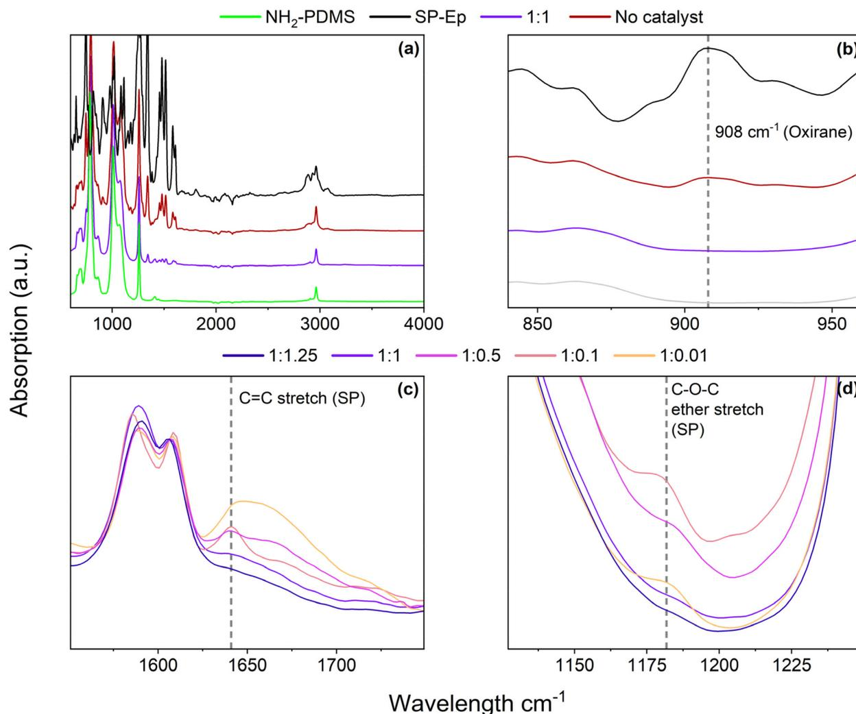
**Fig. 1** (a) IR spectra of PDMS-NH<sub>2</sub>, SP-Ep, and SMP 1:1 with equimolar amount of SP-Ep to ZnCl<sub>2</sub> and sample 1:0 without ZnCl<sub>2</sub>. (b) the functionalization of PDMS-NH<sub>2</sub> with SP-Ep is confirmed by the disappearance of the peak at 908 cm<sup>-1</sup> characteristic of NH<sub>2</sub> groups. (c) and (d) Effect of ZnCl<sub>2</sub> on the isomeric state of SP-Ep is demonstrated by the differences in the IR spectra of the SP and MC forms.
