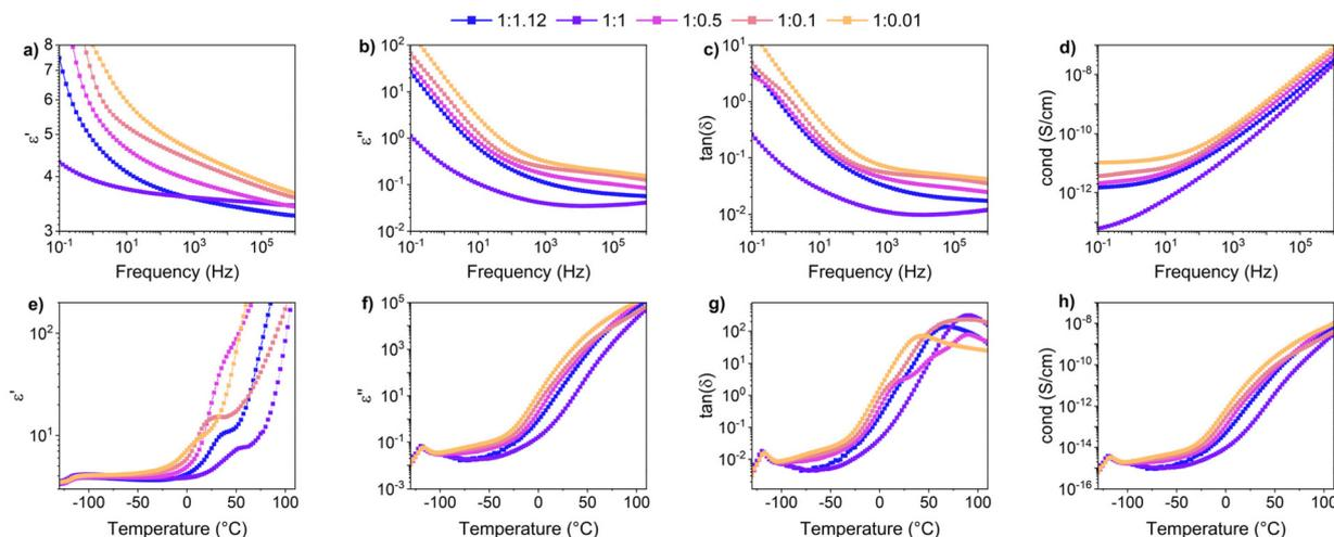
**Fig. 4** Dielectric spectroscopy measurements of samples with different amounts of  $\text{ZnCl}_2$  and pure ligand. Given are the frequency-dependent changes in dielectric permittivity ( $\epsilon'$ ) (a), dielectric loss ( $\epsilon''$ ) (b), dissipation factor ( $\tan \delta$ ) (c), and conductivity (d). (e)–(h) show the temperature-dependent changes in  $\epsilon'$  (e),  $\epsilon''$  (f),  $\tan \delta$  (g), and conductivity (h) at 0.1 Hz.
