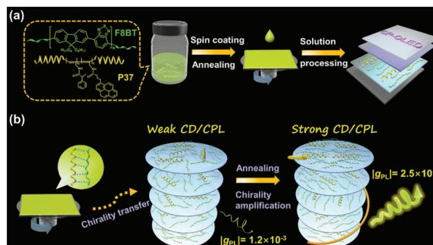
**Fig. 14** (a) Chemical structures of F8BT and P37. (b) The mechanism of F8BT induced by P37. Reproduced with permission.<sup>23</sup> Copyright 2024, Wiley-VCH.
