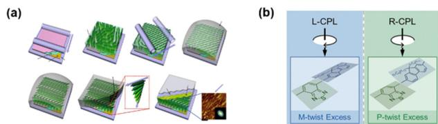
**Fig. 15** (a) Schematic diagrams of the fabrication process. Reproduced with permission.<sup>64</sup> Copyright 2019, Springer Nature (b) scheme depicting the chirality induction of F6BT by left-handed circularly polarized light (L-CPL) and right-handed circularly polarized light (R-CPL), respectively. Reproduced with permission.<sup>65</sup> Copyright 2020, Royal Society of Chemistry.
