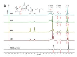
Fig. 1  $\,^{1}$ H NMR spectra of the final purified polymers before (pristine PEtOx) and after reaction at various LR: PEtOx molar ratios: (A) up to 0.15, dissolved in CDCl<sub>3</sub> and (B) from 0.165 on dissolved in TFA-d (LR' stands for the LR-derived thionation by-product).
