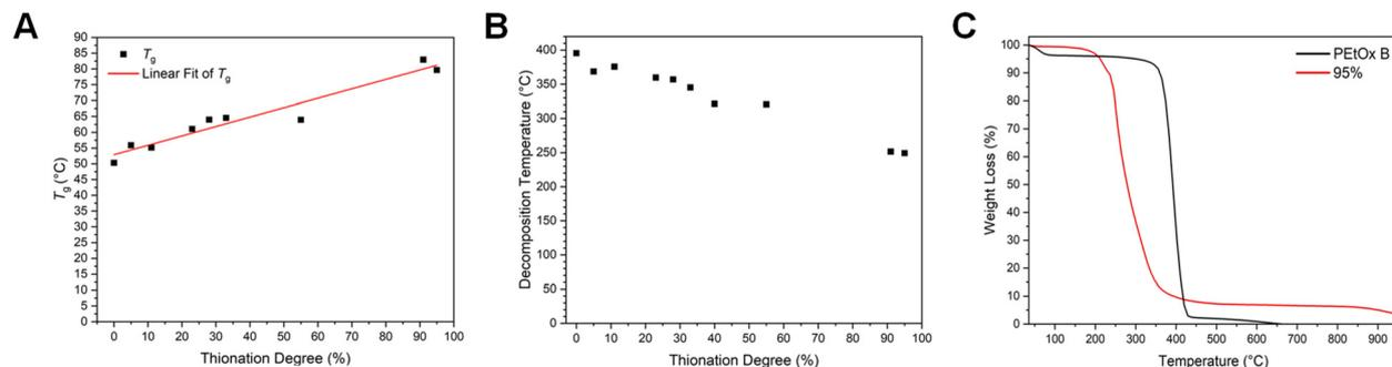
Fig. 4 Variation of the glass transition temperature ( $T_g$ ) (A) and the temperature of maximum weight loss (B) with respect to the thionation degree. (C) TGA thermograms of PETox B and its product of reaction with LR at LR : PETox = 0.5.
