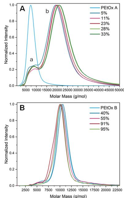
**Fig. 3** SEC chromatograms of pristine PEtOx and PETThz-*co*-PEtOx copolymers with various thionation degrees. (A) Chromatograms in DMAc with 0.7 wt% LiBr. Peak a corresponds to the chains that did not undergo disulfide bridge formation, while peak b corresponds to the dimers after the disulfide bridge formation. (B) Chromatograms in HFIP.
