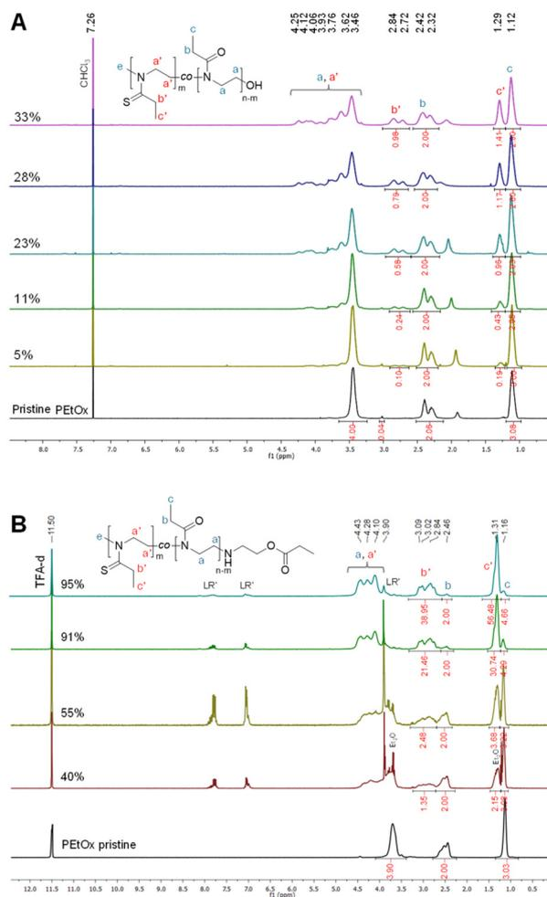
**Fig. 1** <sup>1</sup>H NMR spectra of the final purified polymers before (pristine PEtOx) and after reaction at various LR:PEtOx molar ratios: (A) up to 0.15, dissolved in CDCl<sub>3</sub> and (B) from 0.165 on dissolved in TFA-*d* (LR' stands for the LR-derived thionation by-product).
