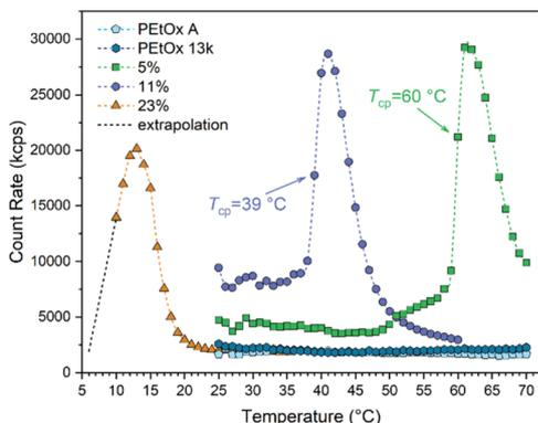
Fig. 5 Evolution of the scattered light intensity for 5 mg mL<sup>-1</sup> aqueous solutions of PEtOx and PEtThz-*co*-PEtOx during heating between 10 and 70 °C at a rate of 1 °C min<sup>-1</sup>.
