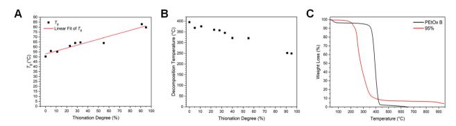
Fig. 4 Variation of the glass transition temperature  $(T_0)$  (A) and the temperature of maximum weight loss (B) with respect to the thionation degree. (C) TGA thermograms of PEtOx B and its product of reaction with LR at LR: PEtOx = 0.5.
