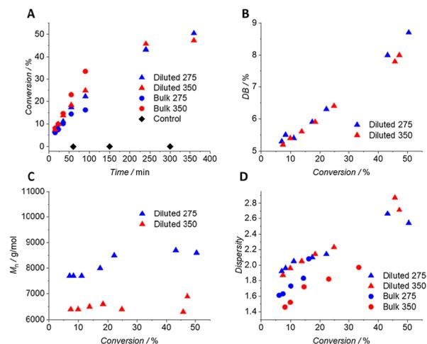
**Fig. 3** Kinetic studies of the RROP of MTC under UV light of 275 and 350 nm at room temperature entailing (A) MTC conversion vs. time development for all kinetics together with control samples kept under light exclusion; (B) DB vs. MTC conversion development for 1 : 1 diluted kinetics; (C) relatively determined  $M_n$  vs. MTC conversion development for 1 : 1 diluted kinetics; and (D) dispersity vs. MTC conversion correlation for all kinetics.
