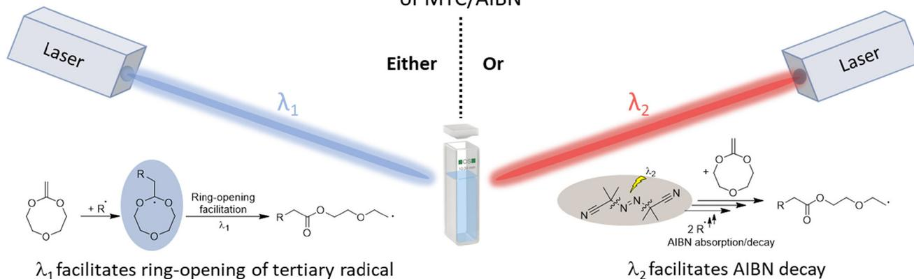
**Scheme 1** AIBN-initiated RROP of MTC exhibits a wavelength-orthogonal behaviour established by photochemical action plot measurements, *i.e.* either enhancement of the ring-opening propensity of the tertiary radical intermediate at  $\lambda_1 = 275$  nm (blue) or photolytic AIBN decay at  $\lambda_2 = 350$  nm (red).
