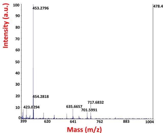
Fig. 3 MALDI-TOF mass spectrum of alanine-coated IONPs.
