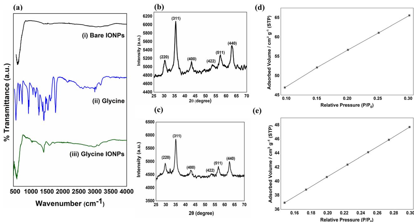
**Fig. 1** Characterization of bare IONPs and glycine-coated IONPs: (a) FTIR spectra of bare IONPs (i), glycine (ii), and glycine IONPs (iii). XRD patterns of (b) bare IONPs and (c) glycine IONPs. Multi-point BET plots of (d) bare IONPs and (e) glycine IONPs.
