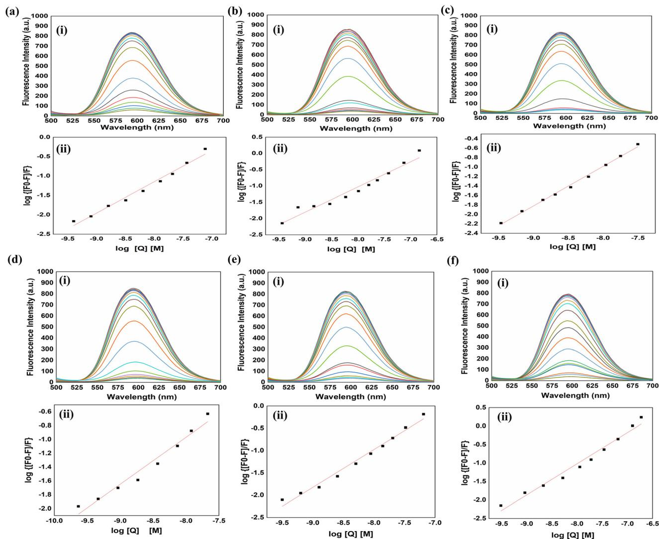
**Fig. 6** Fluorescence emission quenching graph of the complex formed by DNA-EtBr with increasing concentration of the synthesized amino acid-coated IONPs: (a) glycine-coated IONPs; (b) alanine-coated IONPs; (c) aspartic acid-coated IONPs; (d) tryptophan-coated IONPs; (e) serine-coated IONPs; (f) threonine-coated IONPs.
