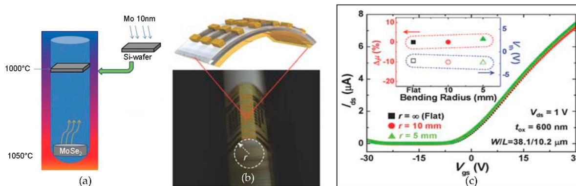
**Fig. 6** High-mobility transistors based on chemical vapor deposition (CVD)-grown MoSe<sub>2</sub>; (a) schematic of the synthesis of MoSe<sub>2</sub> film with modified CVD method; (b) optical image of bended MoSe<sub>2</sub> transistor; and (c) *I*-*V* characteristic of unbent and bent (up to 5 mm of radius) MoSe<sub>2</sub> transistor. Reproduced from ref. 50 with permission from John Wiley and Sons, 2016.
