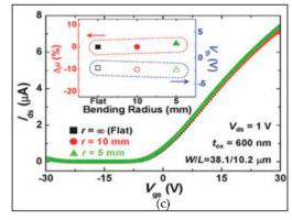
Fig. 6 High-mobility transistors based on chemical vapor deposition (CVD)-grown MoSe<sub>2</sub>; (a) schematic of the synthesis of MoSe<sub>2</sub> film with modified CVD method; (b) optical image of bended MoSe<sub>2</sub> transistor; and (c) *I–V* characteristic of unbent and bent (up to 5 mm of radius) MoSe<sub>2</sub> transistor. Reproduced from ref. 50 with permission from John Wiley and Sons, 2016.
