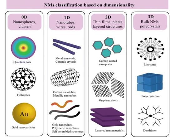
Fig. 3 Schematic of nanoparticles by dimensionality with examples: 0D (nanoparticles), 1D (nanorods), 2D (films), and 3D nanocomposites, where synergistic properties emerge from distinct materials combined at the nanoscale. Reproduced from an open access article, ref. 44 with permission from the Royal Society of Chemistry, 2024.
