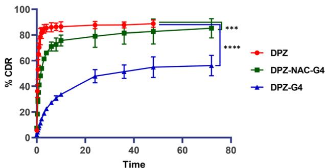
**Fig. 8** *In vitro* release profiles of DPZ from DPZ-NAC-G4, DPZ-G4 and pure drug samples in PBS (pH 7.4) at 37 °C (data presented as mean  $\pm$  SD,  $n = 3$ ). Data were analyzed using one-way ANOVA followed by Dunnett's multiple comparisons test (\*\*\*:  $p < 0.001$ ; \*\*\*\*:  $p < 0.0001$ ).
