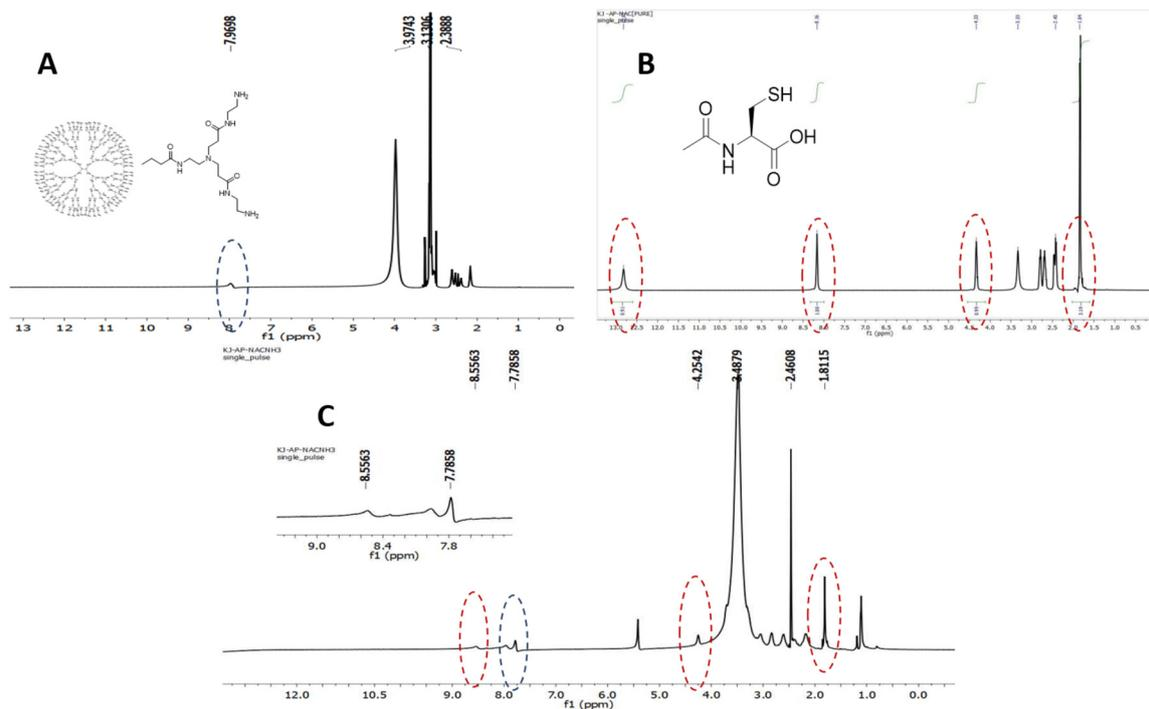
Fig. 4 NMR spectra of PAMAM G4 (A), NAC (B) and the NAC-G4 conjugate (C) in deuterated dimethyl sulfoxide.
