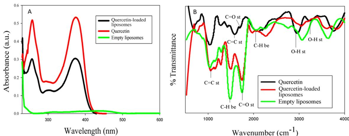
**Fig. 1** (A) UV-visible spectra of quercetin (red curve), quercetin-loaded liposomes (black curve), and empty liposomes (green curve). (B) Fourier transform infrared spectra of free quercetin (black curve), quercetin-loaded liposomes (red curve), and empty liposomes (green curve). “st” stands for stretching and “be” stands for bending.
