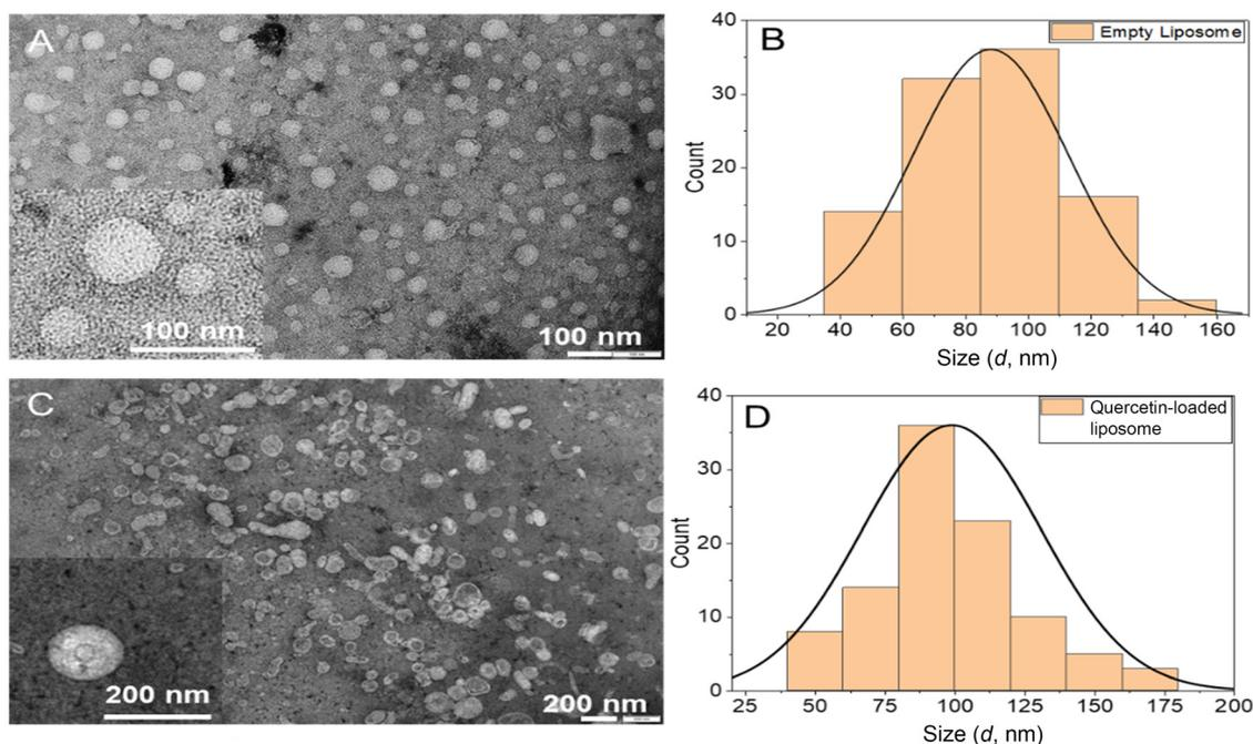
**Fig. 2** Transmission electron microscopy image of empty liposomes (A), particle size distribution of empty liposomes (B), TEM image of quercetin-loaded liposomes (C), and particle size distribution of quercetin-loaded liposomes (D). The insets show high magnification images of the respective liposomes.
