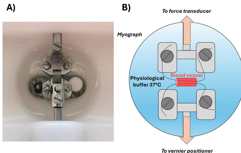
**Fig. 1** Wire myography setup of the *ex vivo* vasodilatory testing using human vascular tissues. (A) Description of wire myography experimental setup. (B) Example of a vessel mounted in a wire myograph and associated schematic representation. Vascular tissue ring (red) was passed through by two tungsten wires which were fixed on transducer jaw for tension measurement. The setup was immersed in physiological bath heated at 37 °C and bubbled with 95% O<sub>2</sub>–5% CO<sub>2</sub> gas mixture.
