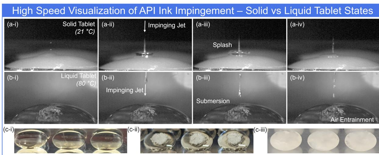
**Fig. 3** High-speed visualization of (a) drop/jet impingement and splashing onto solid tablets and (b) jet impingement and submersion into liquid tablets. Images of  $(1024 \times 576)$  pixels were acquired at 12 000 frames per s by a FASTCAM Nova camera and cropped for display. (c) Photographic images of (i) liquid, (ii) API-dosed, and (iii) solidified tablets. Scale: tablet diameters are approximately 8 mm.
