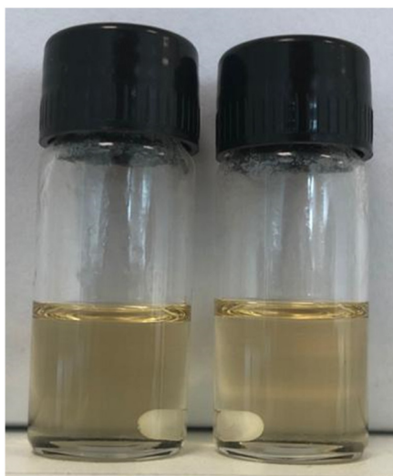
Fig. 2 Developed ME-blank formulation at the final optimized microemulsion composition (% w/w): 10% water, 44% oil mixture (17.8% babassu oil + 26.2% MCT), and 46% surfactant mixture (29.7% Span TM 83 + 7.1% Tween ® 80 + 9.2% Transcutol ® HP) ( n = 2 ) (magnetic bars are inside flasks).
