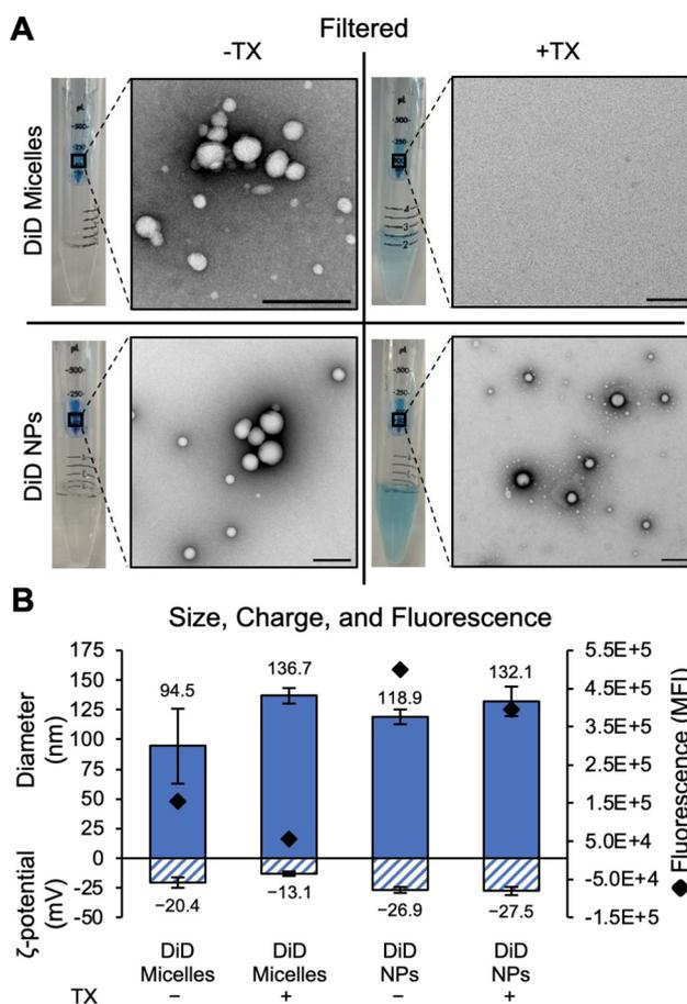
**Fig. 1** Characterization of DiD Micelles and DiD NPs purified by filtering with and without the addition of Triton X-100 (TX). (A) Photographs of filter tubes and representative TEM images (scale bars = 200 nm). (B) Hydrodynamic size, zeta potential, and total fluorescence of each sample.
