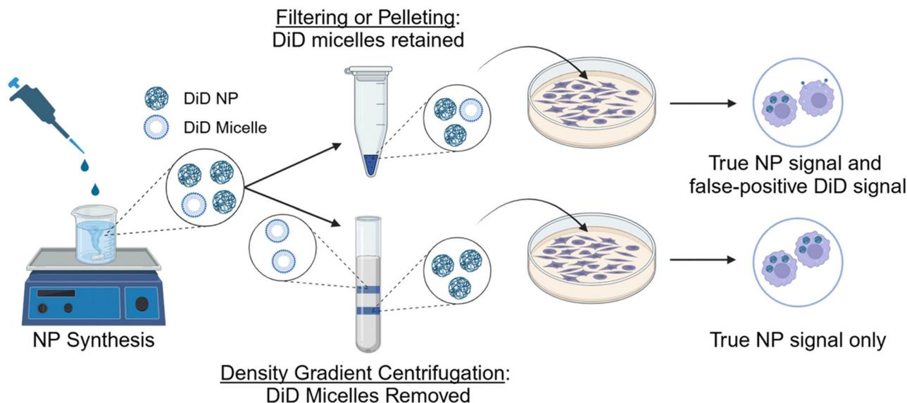
**Scheme 1** Scheme depicting the synthesis of PEG–PLGA NPs encapsulating DiD (DiD NPs) for fluorescence-based trafficking studies. DiD micelles that form in the solution along with the DiD NPs are challenging to remove with conventional purification techniques and can lead to false positive signal. Created with [BioRender.com](#).
