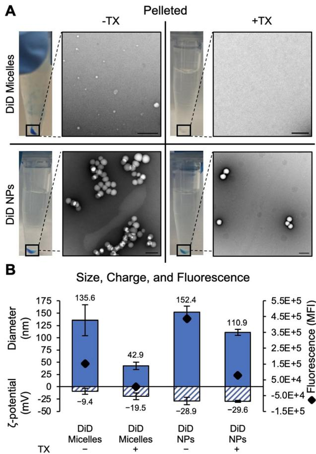
**Fig. 2** Characterization of DiD Micelles and DiD NPs purified by pelleting with and without the addition of TX. (A) Photographs of centrifuge tubes and representative TEM images (scale bars = 200 nm). (B) Hydrodynamic diameter, zeta potential, and total fluorescence of each sample.
