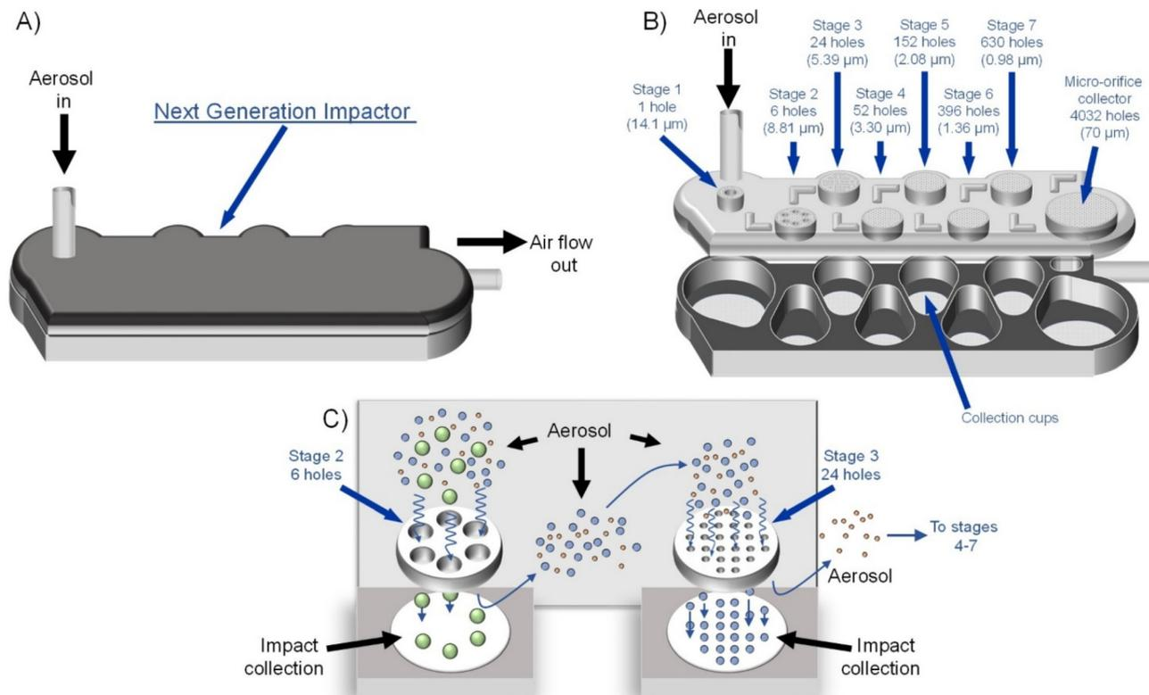
**Fig. 3** Schematic of Next Generation Impactor (NGI) cascade impactor design. (A) The inlet and outlet points, direction of air flow, (B) the locations of the removable collection cups and cut-off sizes of the cup orifices, and (C) a demonstration of aerosolised droplet separation based on size are shown.
