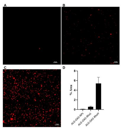
Fig. 5 LSCM images of PLGA NPs in alginate-based biomaterial inks crosslinked with 50 mM CaCl<sub>2</sub> solution (ag.): (A) biomaterial ink 3 (i.e., 9% w/v ALG-OA<sub>5</sub> loaded with 20 mg mL<sup>-1</sup> PLGA NPs); (B) 1 mg mL<sup>-1</sup> Rho-PLGA NPs and (C) 20 mg mL<sup>-1</sup> Rho-PLGA NPs loaded in ALG-OA<sub>5</sub> hydrogels. Scale bars: 10  $\mu$ m. (D) Percentage of area covered by the particles per image. Data are presented as mean  $\pm$  st. dev. (n = 3).
