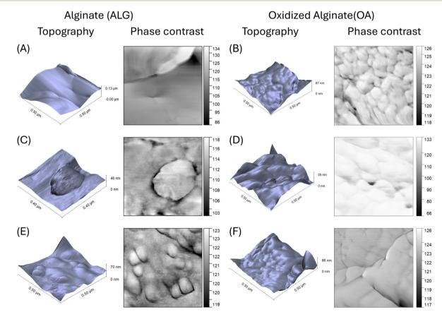
Fig. 4 AFM images of topography and phase contrast images of a 500  $\times$  500 nm scan area of: (A) ALG; (B) OA<sub>5</sub>; (C) ALG-PLGA NPs; (D) OA<sub>5</sub>-PLGA NPs; (E) ALG-CS/PLGA NPs; and (F) OA<sub>5</sub>-CS/PLGA NPs.
