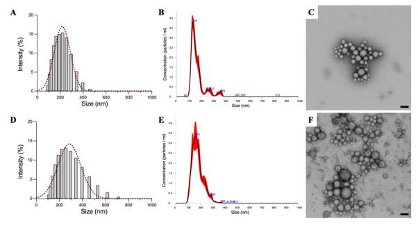
Fig. 1 Characterization of PLGA NPs: (A) DLS size distribution (grey bars) and fitting (red dotted line), (B) NanoSight size analysis, and (C) TEM micrographs. Characterization of CS/PLGA NPs: (D) DLS size distribution (grey bars) and fitting (red dotted line), (E) NanoSight size analysis, and (F) TEM micrographs. NPs were prepared with microfluidics and then coated using 0.1% w/v chitosan in 4.6 mM HCl (aq.) solution. TEM image scale bars: 200 nm.
