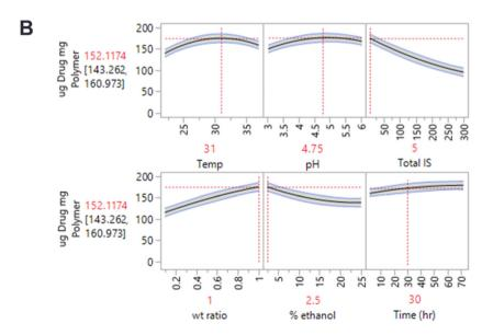
Fig. 2 Summary of conditions to maximize the loading of paclitaxel and carboplatin into P(DEAEMA-co-CHMA)-g-PEGMA nanogels. Data was analyzed in JMP software. (A) Actual versus predicated values for mass of API loaded per mass of nanoparticle with an R-square value of 0.98 (p < 0.0001). (B) Resulting predication profiler showing maximal loading conditions.
