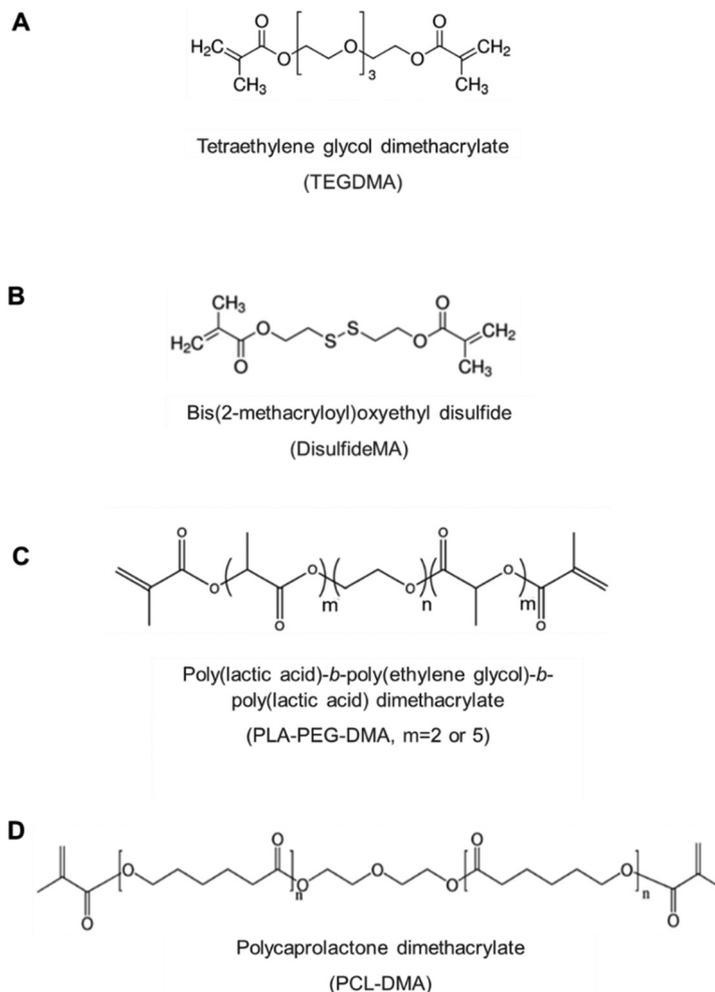
**Fig. 1** Structures of degradable crosslinking agents investigated. (A) A disulfide crosslinking agent that can be reduced in the presence of intracellular glutathione, and (B–D) three ester-labile crosslinking agents that can be degraded by the presence of intracellular carboxylesterase.
