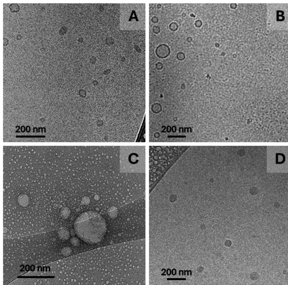
**Fig. 3** Cryo-TEM images for (A) Chol-PEO<sub>22</sub>-N<sub>3</sub> and (B) Chol-PEO<sub>22</sub>-N<sub>3</sub> NPs loaded with 5% w/w UA, (C) Chol-PEO<sub>22</sub>-GlcNAc and (D) Chol-PEO<sub>22</sub>-GlcNAc NPs loaded with 5% w/w UA. The value of 5% w/w refers to the UA feeding.
