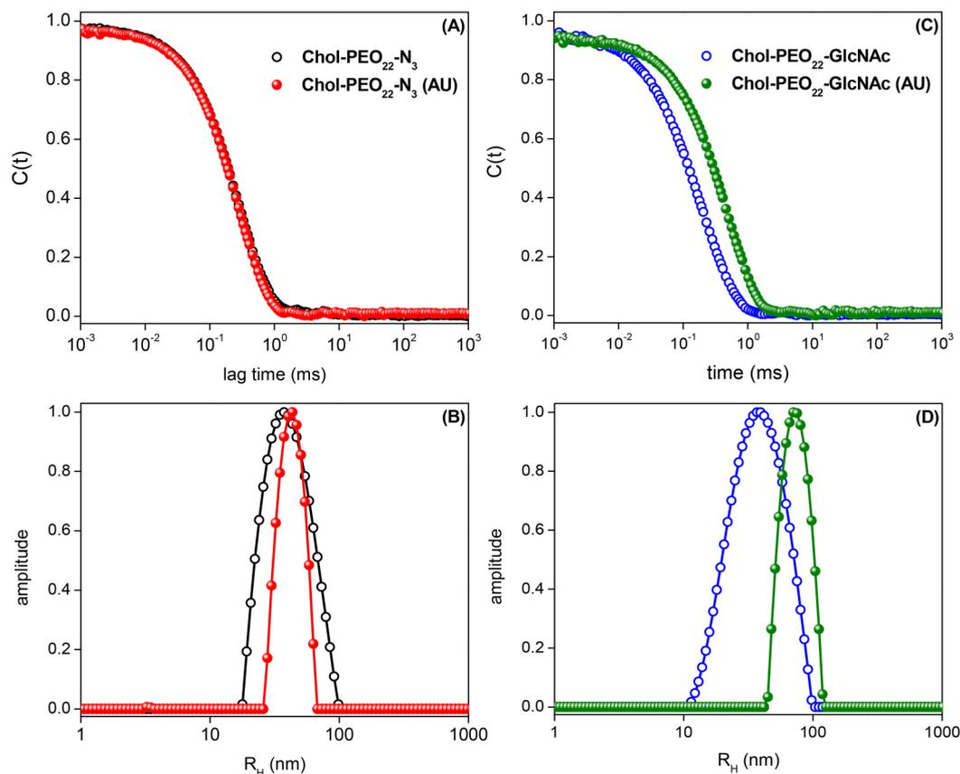
**Fig. 2** Dynamic light scattering data acquired for drug-free and 5% w/w UA-loaded Chol-PEO<sub>22</sub>-N<sub>3</sub> and Chol-PEO<sub>22</sub>-GlcNAc NPs: (A and C) auto-correlation functions and (B and D) respective distributions of sizes.
