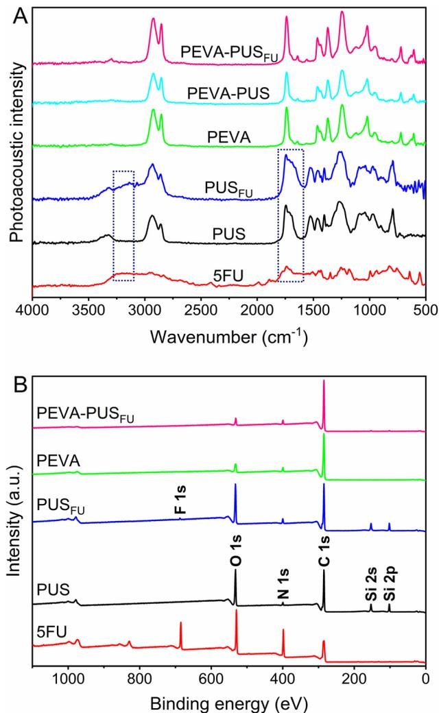
**Fig. 2** (A) Fourier transform infrared photoacoustic spectra of pure 5FU and polymer coatings as indicated; the dashed boxes highlight peak broadening resulting from the inclusion of 5FU within the PUS matrix. (B) X-ray photoelectron spectroscopy survey spectra recorded for pure 5FU and polymer coatings as indicated.
