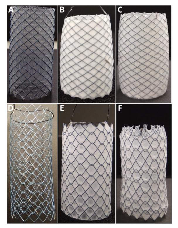
Fig. 1 (A) Membrane-covered OS with fixed braided cell structure and its (B) PUS<sub>FU</sub> and (C) PEVA-PUS<sub>FU</sub> coated derivatives. (D) Bare CS with unfixed woven cell structure and its (E) PUS<sub>FU</sub> and (F) PEVA-PUS<sub>FU</sub> coated derivatives.
