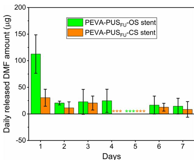
Fig. 7 Amount of residual dimethylformamide (DMF) released from PEVA-PUS<sub>FU</sub>-OS and -CS as a function of time. Three asterisks (\*\*\*) indicate the amount of DMF that was below the quantitation limit (5 ppm). Data are expressed as mean ( $n = 3$ ) ± SD.
