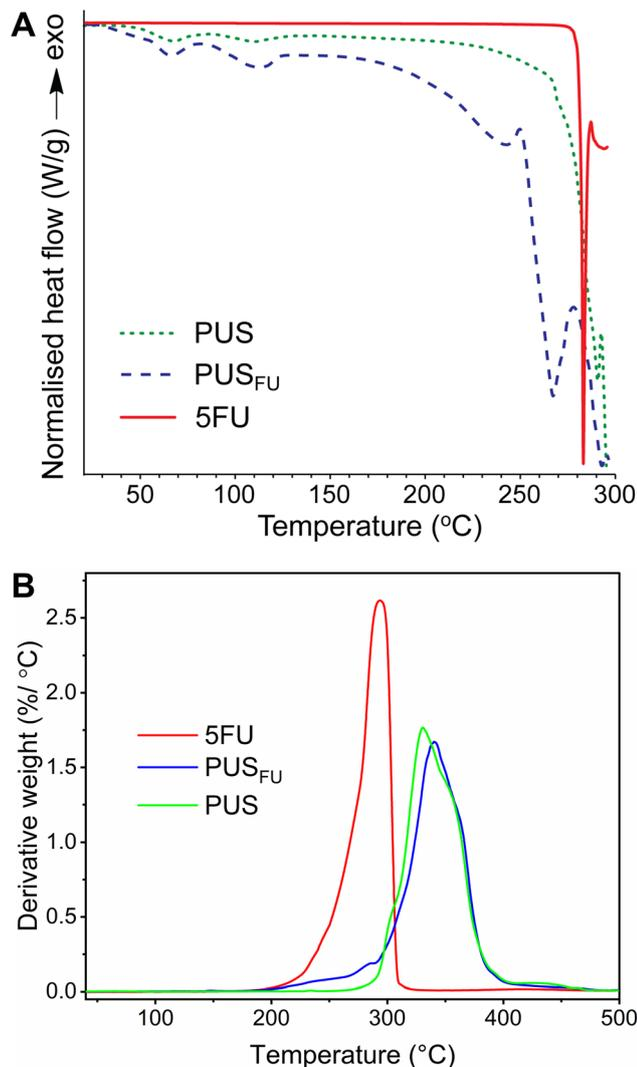
**Fig. 4** (A) Modulated differential scanning calorimetry thermograms recorded at a heating rate of  $2\text{ °C min}^{-1}$  and (B) derivative thermogravimetric curves recorded at a heating rate of  $10\text{ °C min}^{-1}$  for pure 5FU, and  $\text{PUS}_{\text{FU}}$  and PUS coatings.
