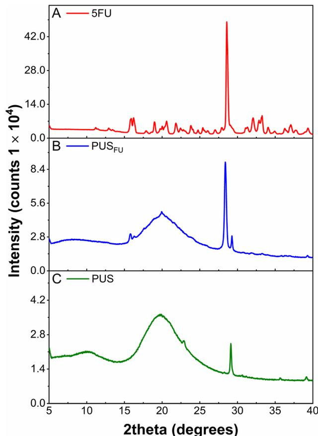
**Fig. 3** X-ray diffractograms of (A) pure 5FU, and (B) **PUS<sub>FU</sub>** and (C) **PUS** coatings.
