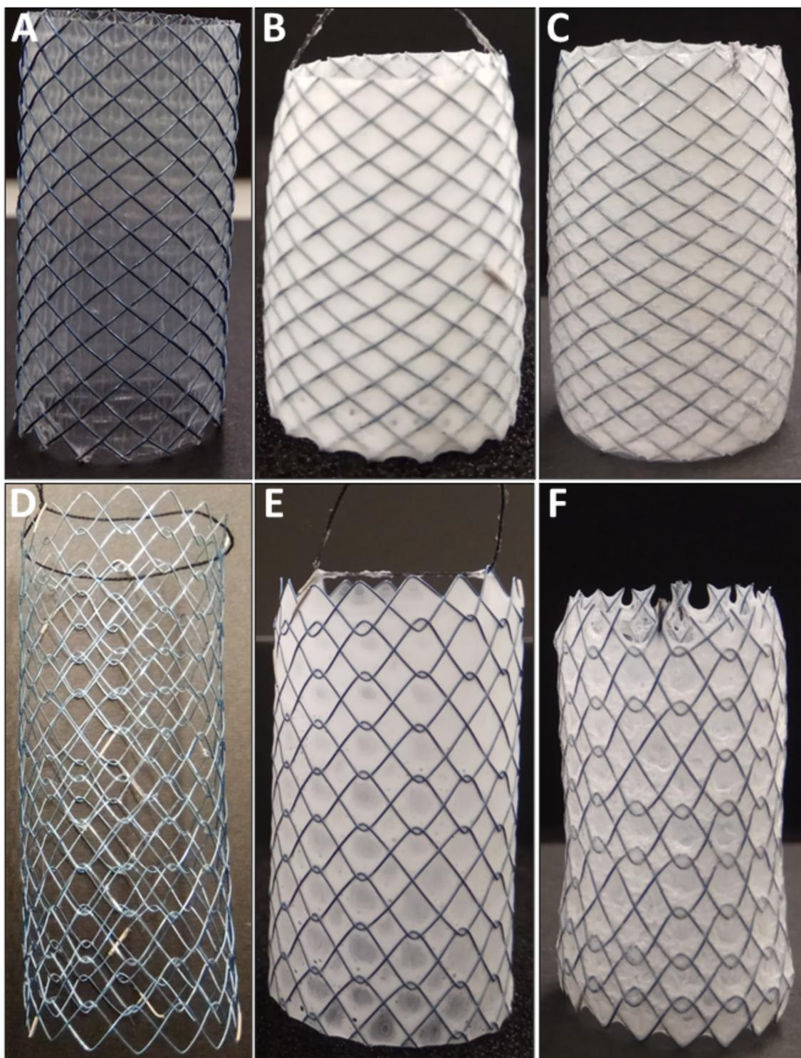
**Fig. 1** (A) Membrane-covered OS with fixed braided cell structure and its (B)  $\text{PUS}_{\text{FU}}$  and (C)  $\text{PEVA-PUS}_{\text{FU}}$  coated derivatives. (D) Bare CS with unfixed woven cell structure and its (E)  $\text{PUS}_{\text{FU}}$  and (F)  $\text{PEVA-PUS}_{\text{FU}}$  coated derivatives.
