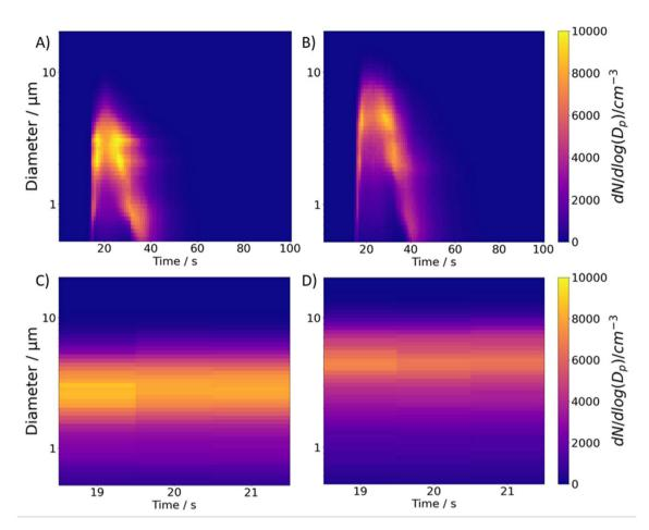
Fig. 1 Plume development in an initial formulation of 3%w/w mannitol actuated from a nebulizer over 3 seconds of actuation at (A) 52% RH in APS<sub>dry</sub> and (B) 95% RH in APS<sub>wet</sub>. (C) and (D) show the first 3 stable seconds for lower and higher RH, respectively.
