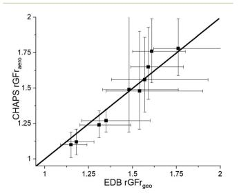
Fig. 6 Comparison between the CK-EDB rGFr<sub>qeo</sub> of aqueous trehalose and the CHAPS rGFraero
